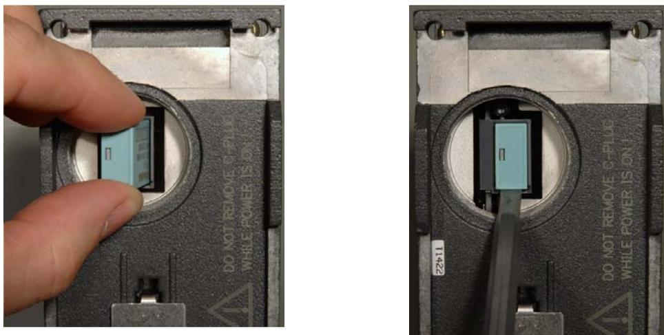
Figure 2-6 Inserting the C-PLUG in the device and removing the C-PLUG from the device with a screwdriver
