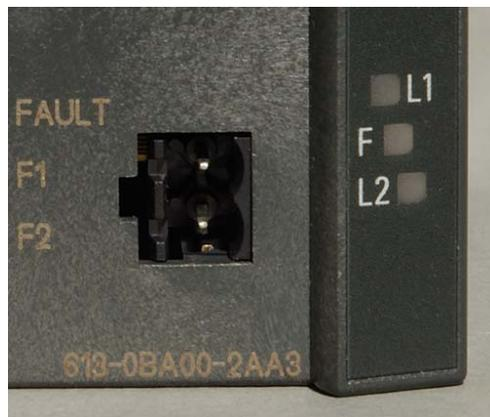
Figure 2-2 Signaling contact
