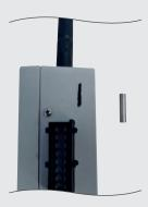
Follow the installation manual for the receivers and install the wire harness to connect the receiver to the PWC. At this time do not fix the receiver to the gastank, cause you have to programm the number of the PWC to the receiver, as soon as it is connected to power.
