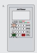
2. To unlock the PWC you have to switch on the remotecontrol by pressing »ON« for 3 seconds, after that press the number of the PWC and »ON«. It will appear »sending«. After you unlocked, the client can restart the PWC with the »Start« button on the PWC.
