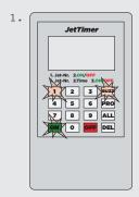
1. To give your client an acoustical signal you have to switch on the remote-control by pressing the "ON" button for 3 sec. Choose the number of PWC, for example "1" press "BUZZ" and then "ON". The client gets a "beep" for 2,5 seconds.
