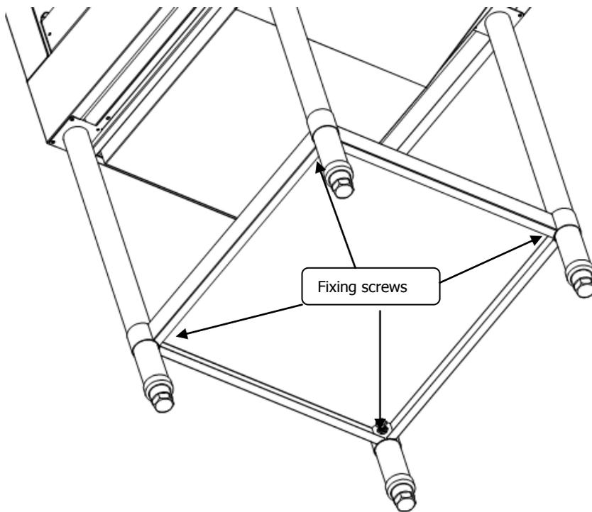
Step 4 – Locate the stand into required position, and adjust the adjustable feet into a level position, refit griddle plate.
