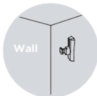
**IMPORTANT NOTICE: Due to a 2-3-sec delay time to record, we recommend to mount the PIR-SD about 15ft from the intended monitoring object for proper recording.**
