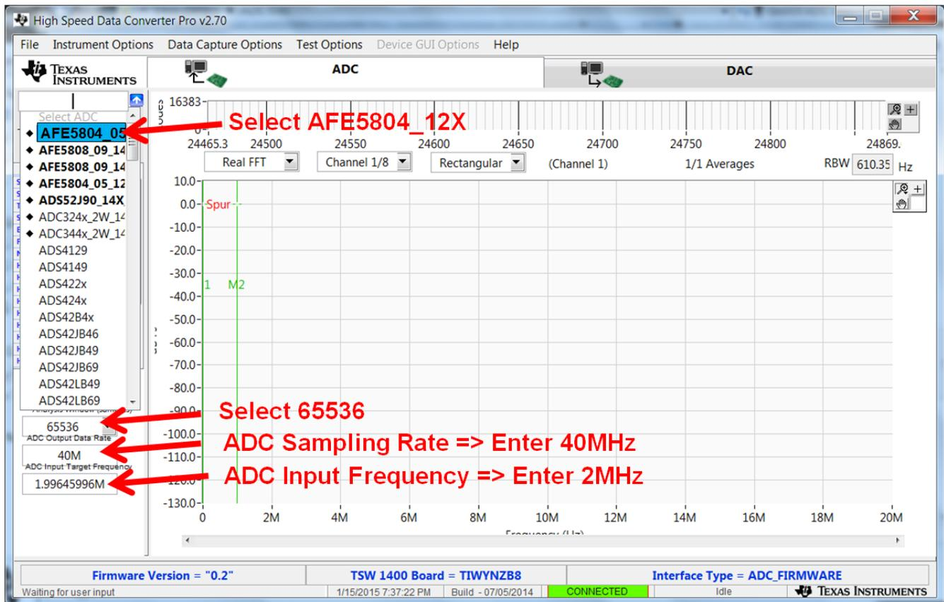
**Figure 19. User Interface: Step-by-Step setup**
