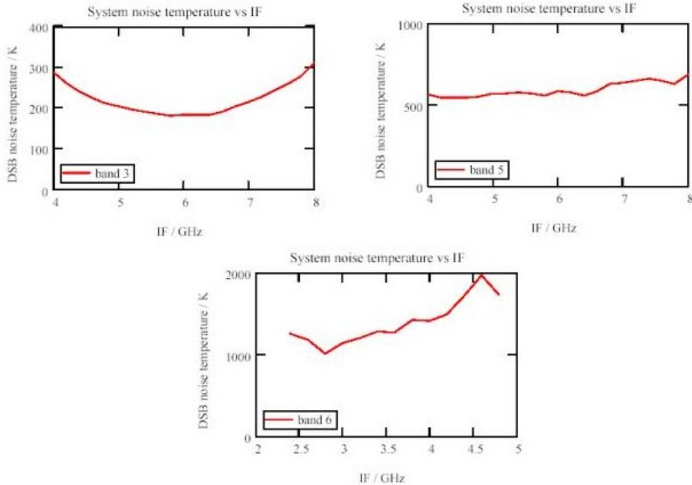
Figure 3.4. Variation of IF sensitivities for band 3, 5 and 6 that show the typical variation of system temperature across the IF band for the diplexer, beamsplitter and high frequency band cases respectively. Note that bands 6 and 7 have a decreasing sensitivity with increasing intermediate frequency.
