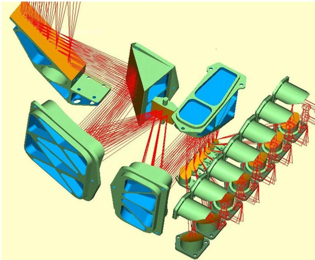
Figure 2.6. HIFI telescope relay optics.
