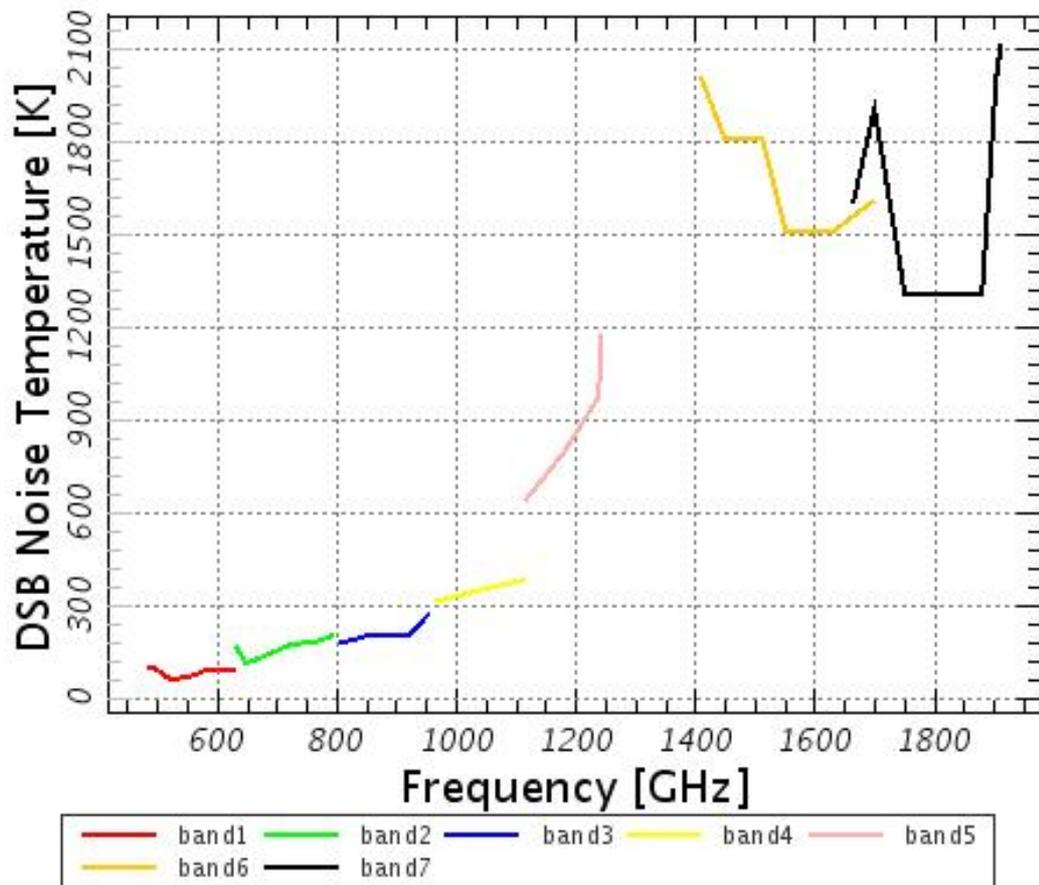
Figure 3.3. Double sideband system temperatures of HIFI mixers (bands 1 to 5 are SIS mixers, bands 6 and 7 are HEB mixers), as used in HSpot. System temperatures are based on ground-based test measurements on the flight model of HIFI.
