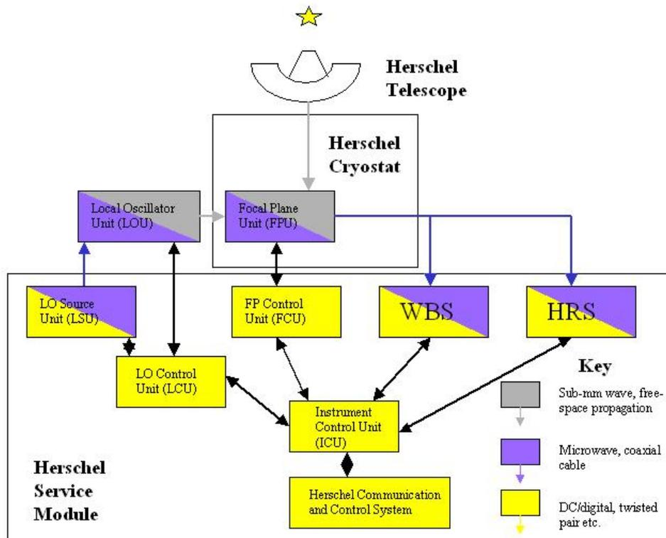
Figure 2.3. General HIFI component diagram.
