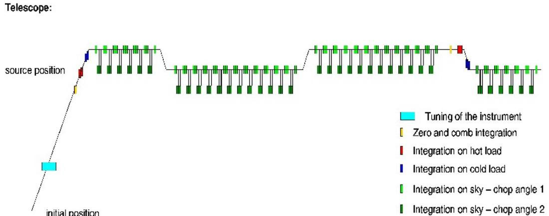
Figure 4.4. Timeline of the HIFI Dual Beam Switch observing mode.
