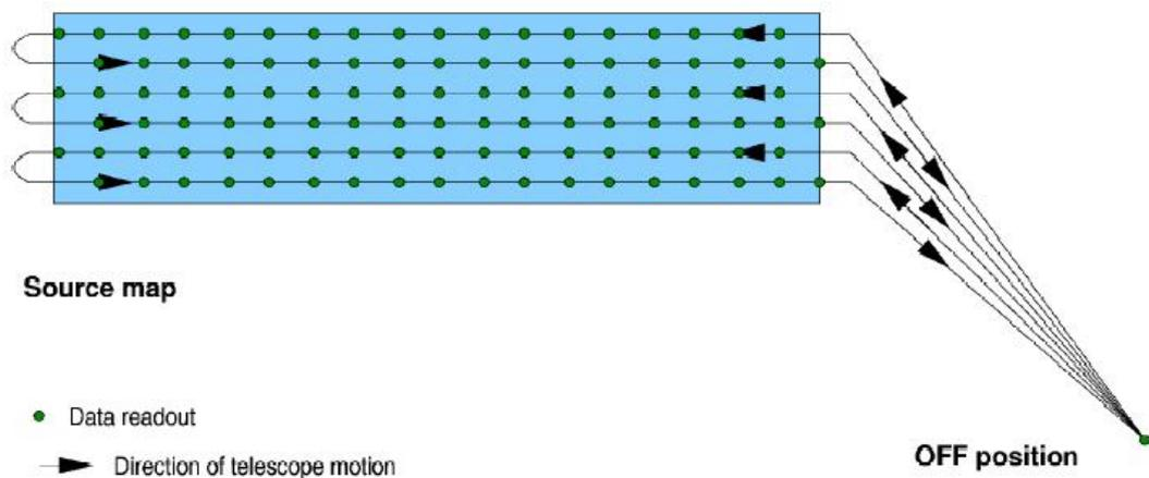
**Figure 4.7. Timeline of the path on the sky for a HIFI OTF mapping mode. The green dots indicate regular data readouts of the spectrometers. The OFF position is returned to at the end of an integer number of scan legs. This is typically 1 or 2 except in the case of small OTF maps.**
