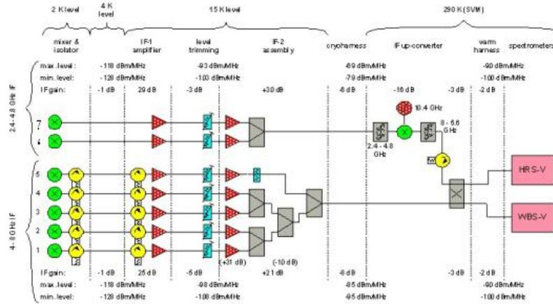
Figure 2.11. The HIFI signal chain.
