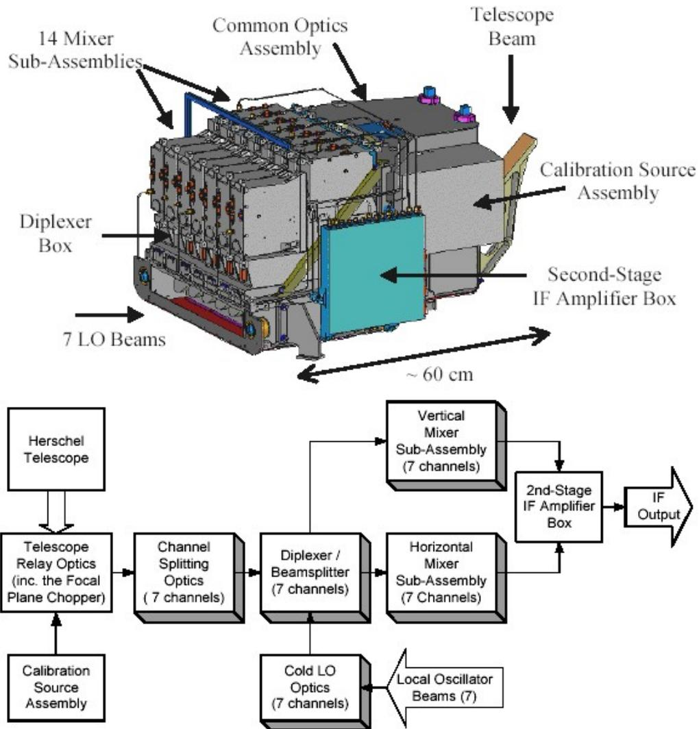
Figure 2.4. HIFI Focal Plane Unit (FPU).
