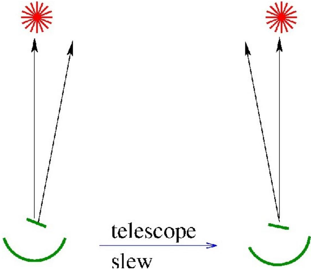
Figure 4.3. HIFI Dual Beam Switch positions on the sky.
