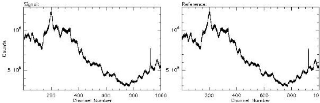
Figure 7.2. Typical level 0 raw data for single dish sub-millimetre signal and reference source scans.
