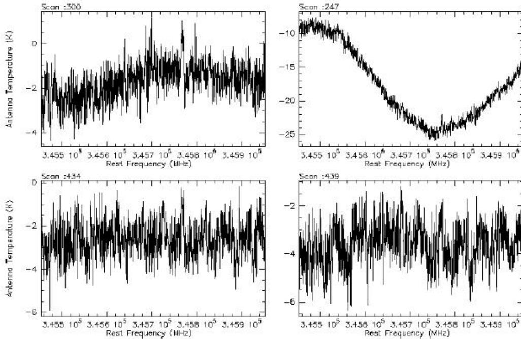
Figure 7.3. Typical level 1 calibrated scans from a single observation showing the different types of baseline problems that can occur in individual scans.
