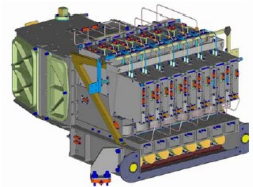
Figure 2.5. Back side of the HIFI FPU.
