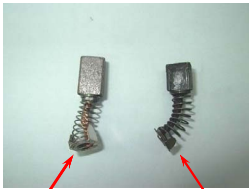
New Motor Brush Worn Motor Brush (Fig 18)
