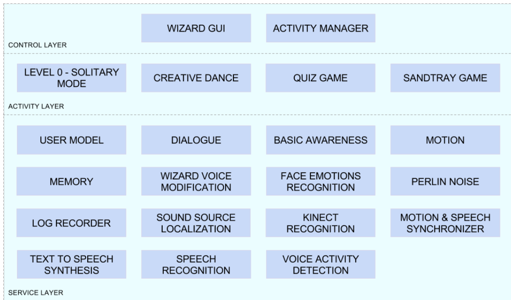
Figure 5: Components of the system organized by functional layers.
