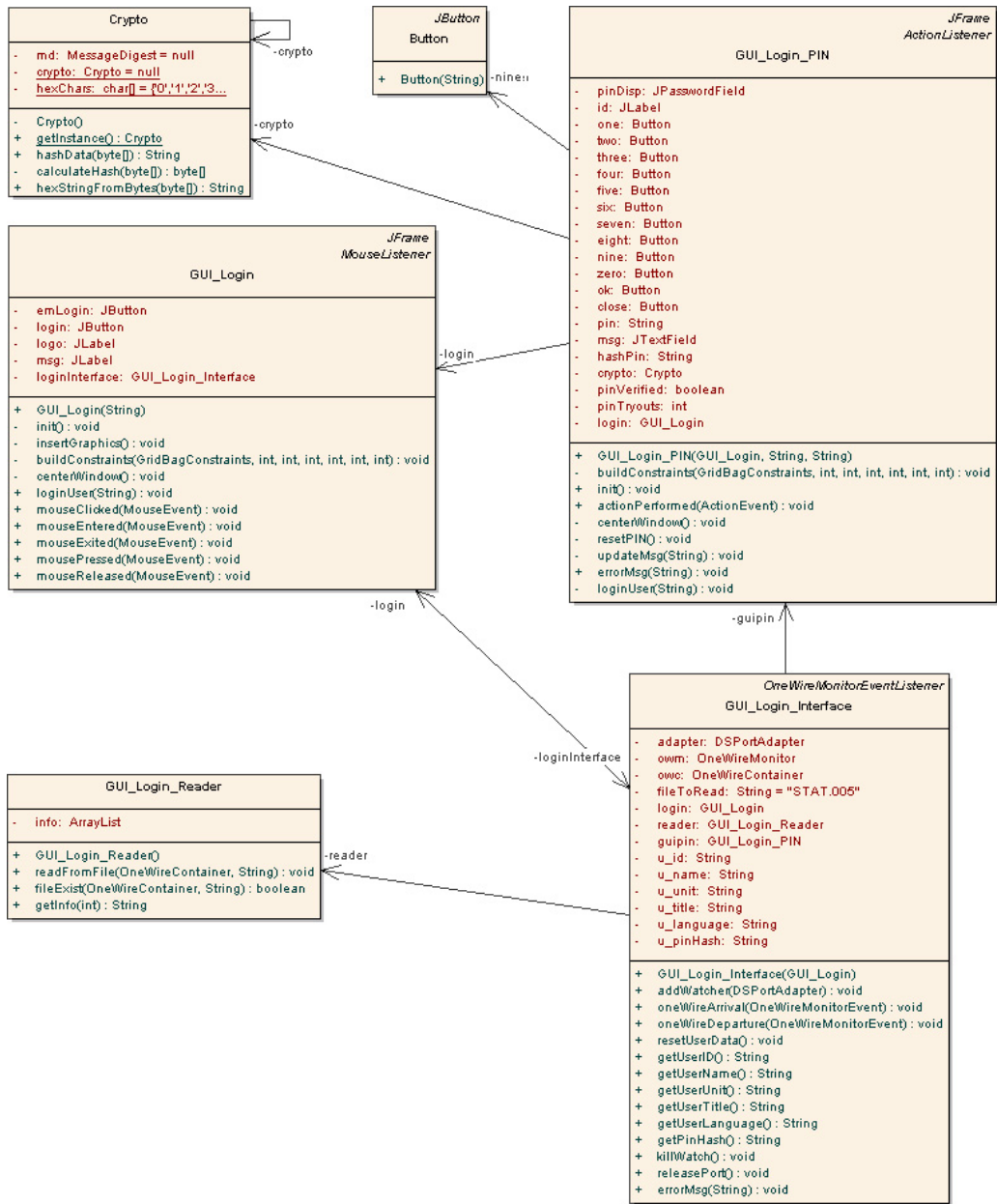
Figure 6.12 – UML class diagram of the new login This diagram shows all the classes with variables and methods in the new login.
