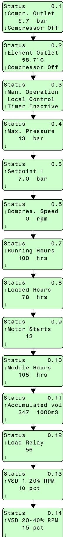
1. **P compressor outlet** : Indication of the pressure read by the sensor in machine outlet
