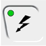
**Power supply indicator** (green lamp lit): controller powered on
