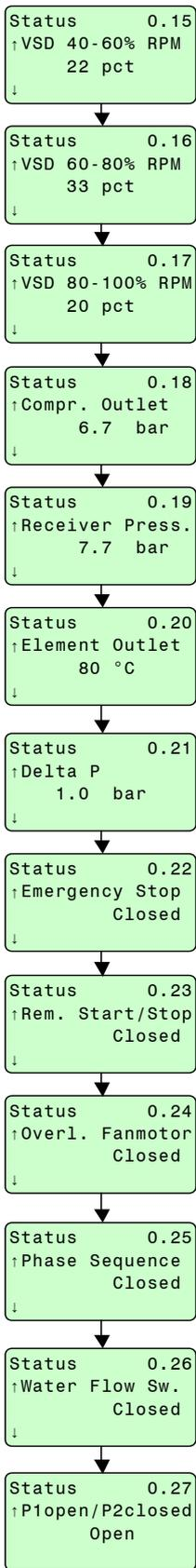
15. **VSD 40-60% RPM** : Percentage of operating time during which the compressor has operated between 40 and 60% of its maximum speed.
