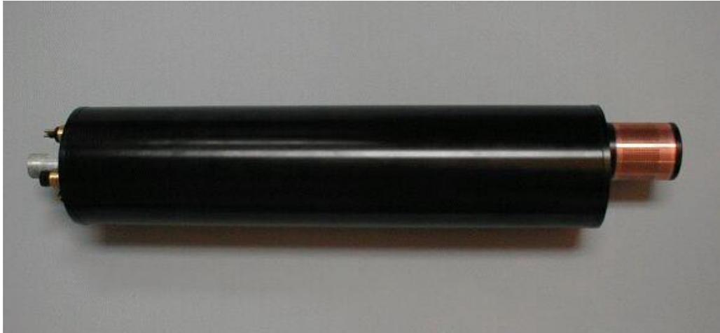
*Figure F-10: The ISUS with Biofouling Guard*
