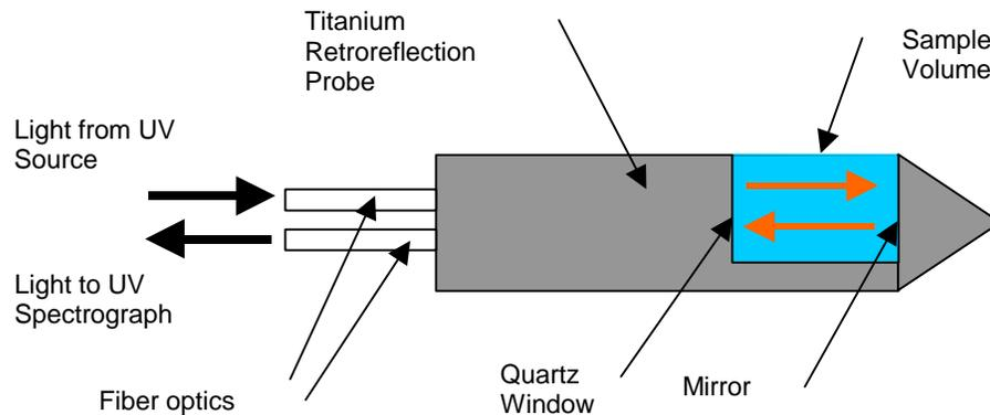
**Figure A-3: Seawater Sample Illumination**
