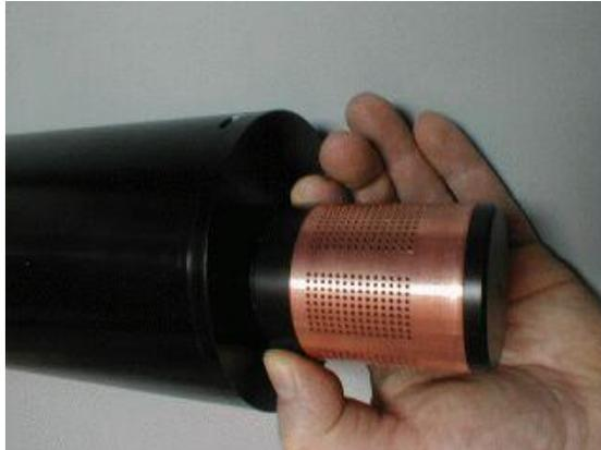
*Figure F-9: Mounting the guard*
