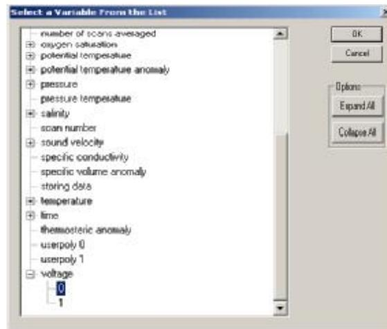
22. On another unused row, click **Select Variable**. From the drop down list, select *voltage 1*. Display 6 decimal places. This is the auxiliary voltage as measured by the CTD.
