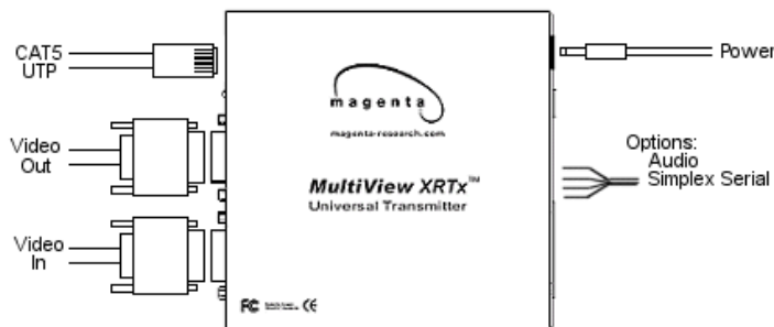
Figure 3-1. Connections on the XRTx Universal Transmitter.
