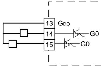
In OP10-230 however, the internal transformer's capacity restricts the current on  $G_{DO}$  to approx. 165 mA.
