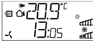
This is an example of the Base Display, the display that is normally shown when there is no operator activity.
