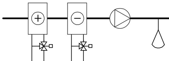
For control mode 2, "Supply air temperature control with outdoor compensation" you need two sensors, "Supply air sensor" on AI1 and "Outdoor sensor" on AI2.
