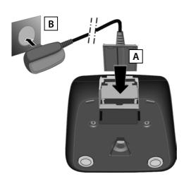
> Place the handset in the charger and wait until the batteries are fully charged (approx. 10 hours).
