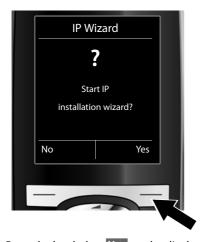
> Press the key below Yes on the display (= right display key).
