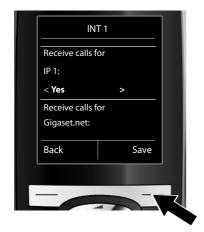
If no calls to the VoIP connection IP 1 are to be signalled on the handset:
