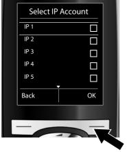
A list of all possible IP connections is shown in the display (IP 1 to IP 6). VoIP connections that are already configured are marked with  $\overline{M}$ .
