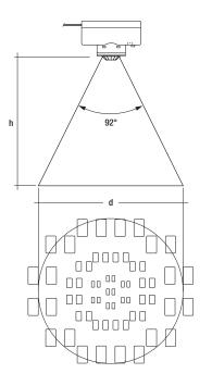
Detection area: 46° Scope: 2.5 m presence detection 5 m motion detection
