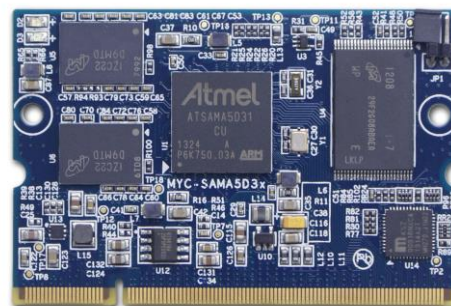
Figure 1-5 MYC-SAMA5D3X CPU Module Controller Board of MYD-SAMA5D3X
