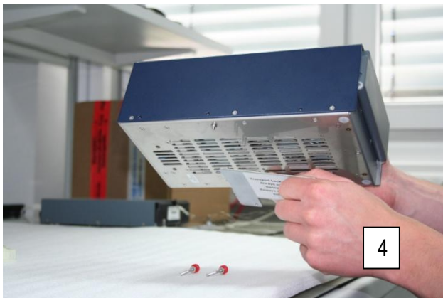
Picture 5: Assembling / disassembling of transportation lock (3 pieces)!
