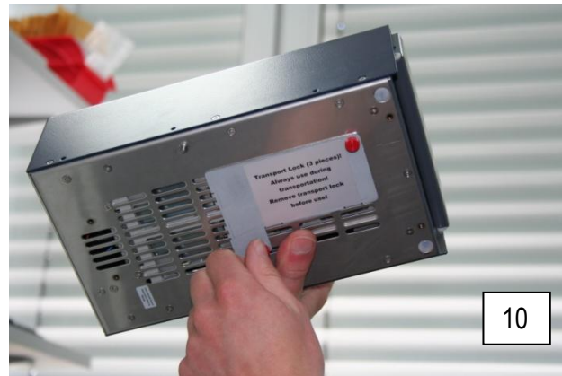
Picture 5.1: Assembling / disassembling of transportation lock (3 pieces)!
