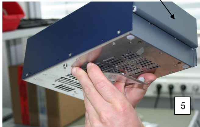
Picture 5: Assembling / disassembling of transportation lock (3 pieces)!
