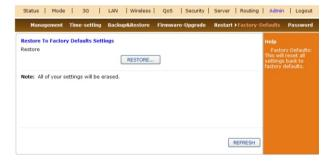
Load Factory Defaults: Click this 'RESTORE...' button to remove all settings you made, and restore the configuration of this router back to factory default settings
