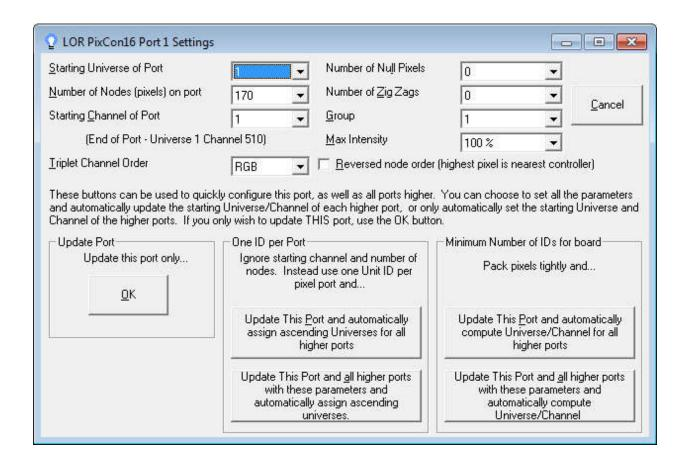
This allows for advanced configuration of the 16 pixel ports. Each port can be individually configured for its start universe, start channel, number of nodes (or pixels), null pixels, zig-zag and reversing.
