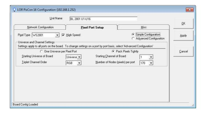
This window allows you to setup the pixel ports on the PixCon16. At a minimum you will need to select the type of pixels you are going to connect, if they are high speed or not, starting universe/unit ID, and the triplet order.
