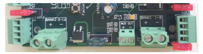
The board can run on any voltage between 5VDC – 30VDC. The voltage you use will be dependent on the type of pixel in use. Power must be supplied from a stable DC source/power supply. The maximum rating of the board is 64A, 32A per bank, 4A per pixel port. Each port is protected by a 4A (pink) blade type fast-blow fuse.
