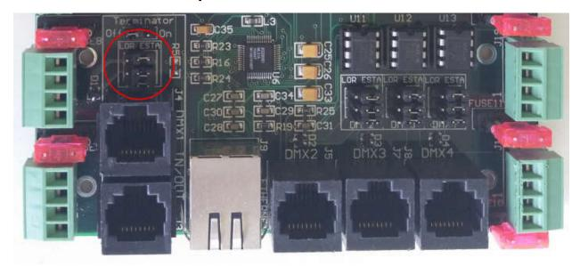
Whenever LOR equipment is in use on any of these RJ45 jacks, the jumpers must be moved from the ESTA side to the LOR side. LOR controllers, even in DMX mode, use a pinout that is different from other devices. Moving these jumpers sets the correct pins.
