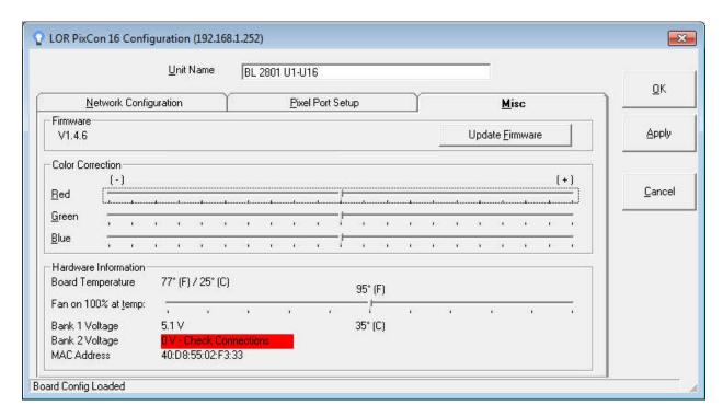
Unit Name is available on all tabs. This allows the user to assign a custom nickname to the controller. The Misc tab allows you to perform a firmware update, change color correction values, set optional fan speed. The board's current information including temperature and operating voltages are shown.
