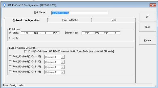
Here you can specify the static IP address and subnet mask that the controller will operate on as well as the type of IP connection. (Use DHCP to instantly see and configure the controller on any existing LAN.)
