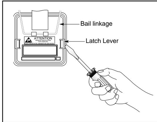
Figure 20-1 Releasing Latch Levers
