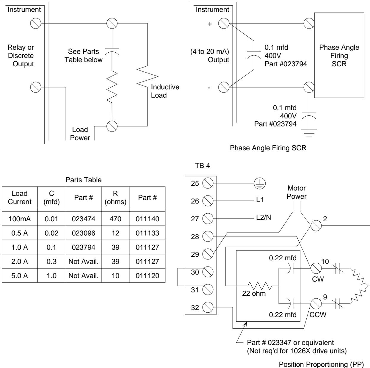
**Figure 4-1 Noise Suppression For Outputs**
