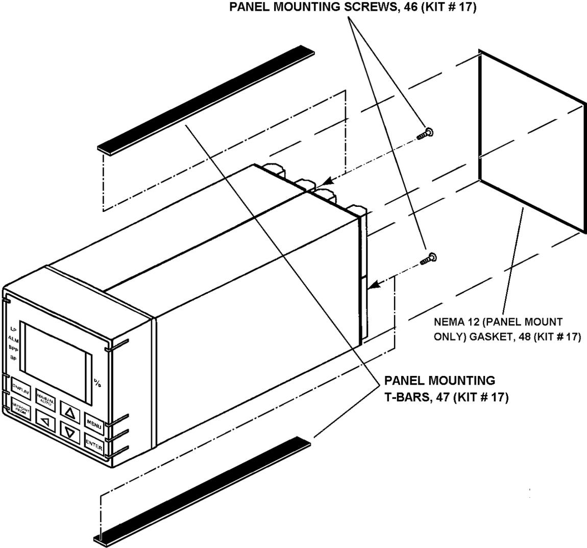
Figure 22-1 Instrument Panel Mounting Hardware
