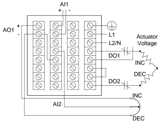
Figure 10-2 Wiring for Factory Configuration 11 (Shown in Figure 10-1)
