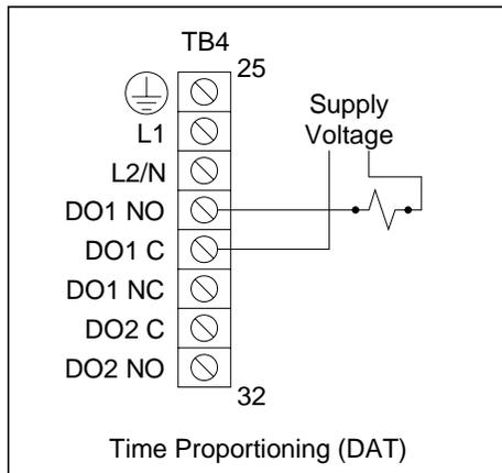
**Figure 4-10 DAT Typical Wiring**
