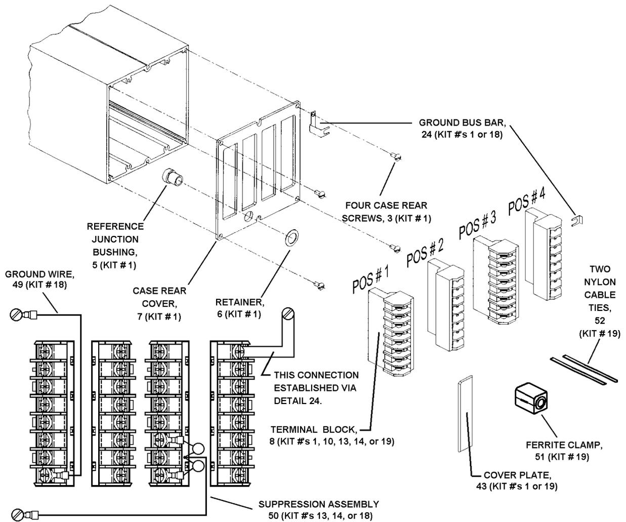
Figure 22-4 Components of Instrument Rear Assembly
