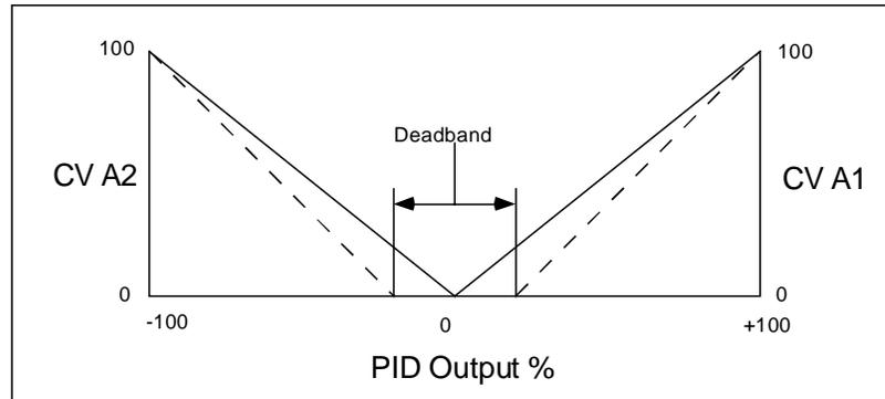
Figure 9-2 CV Standard Split Output Function
