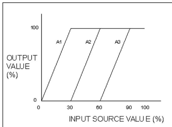
Figure 9-3 CV Advanced Splitter (Default Outputs)
