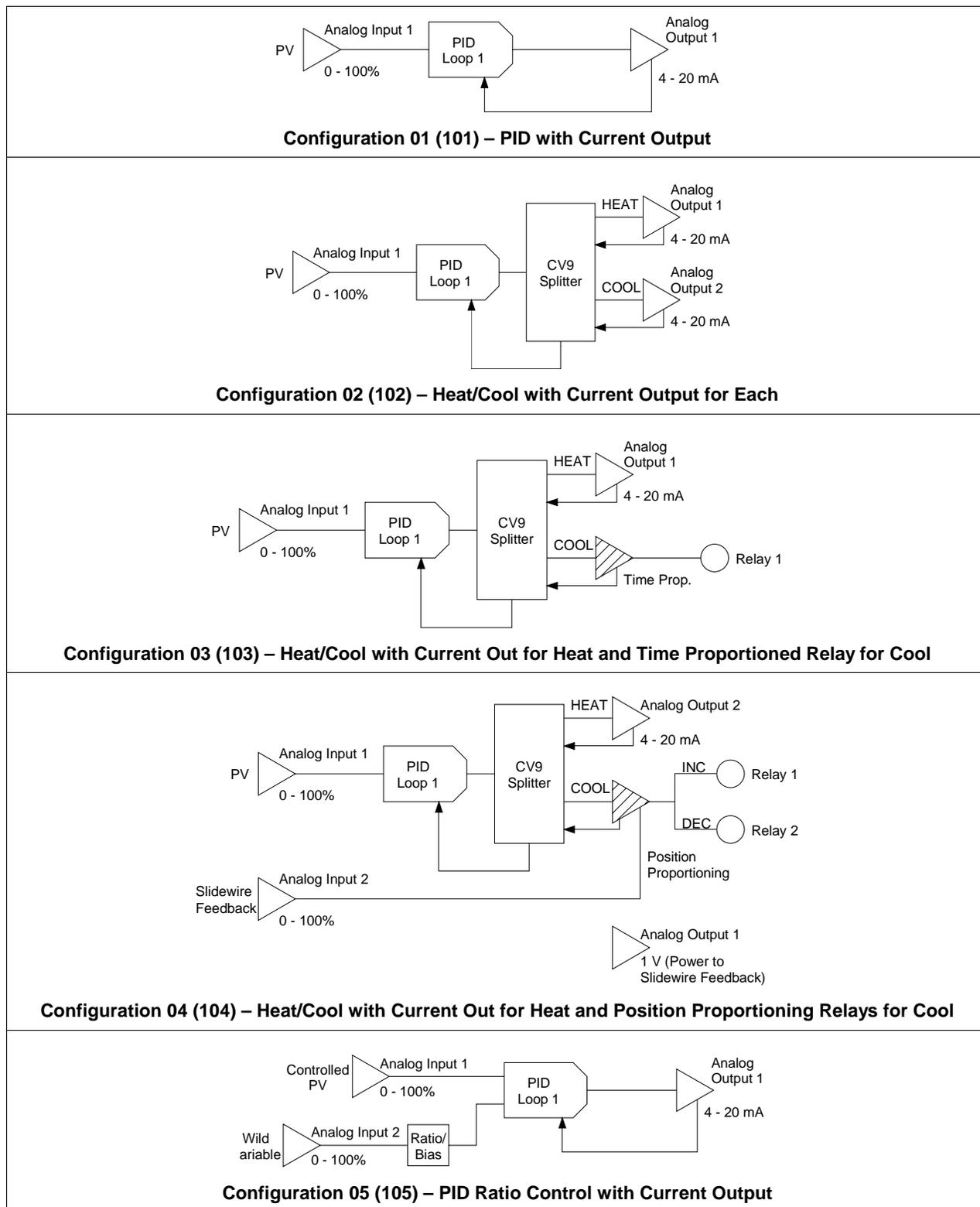
Figure 5-2 Single-Loop Factory Configurations
