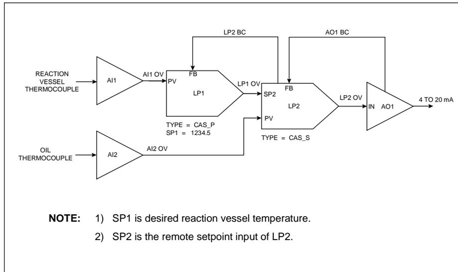
**Figure 8-12 Function Block Diagram of the Cascade Control Strategy**
