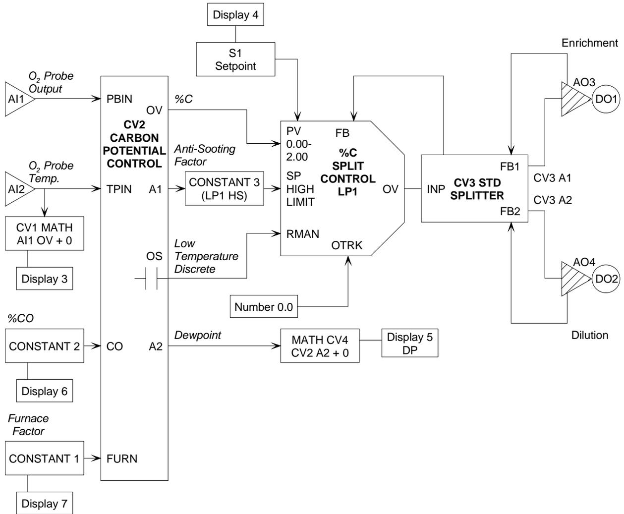
Figure 12-1 Diagram of Carbon Potential Configuration Example
