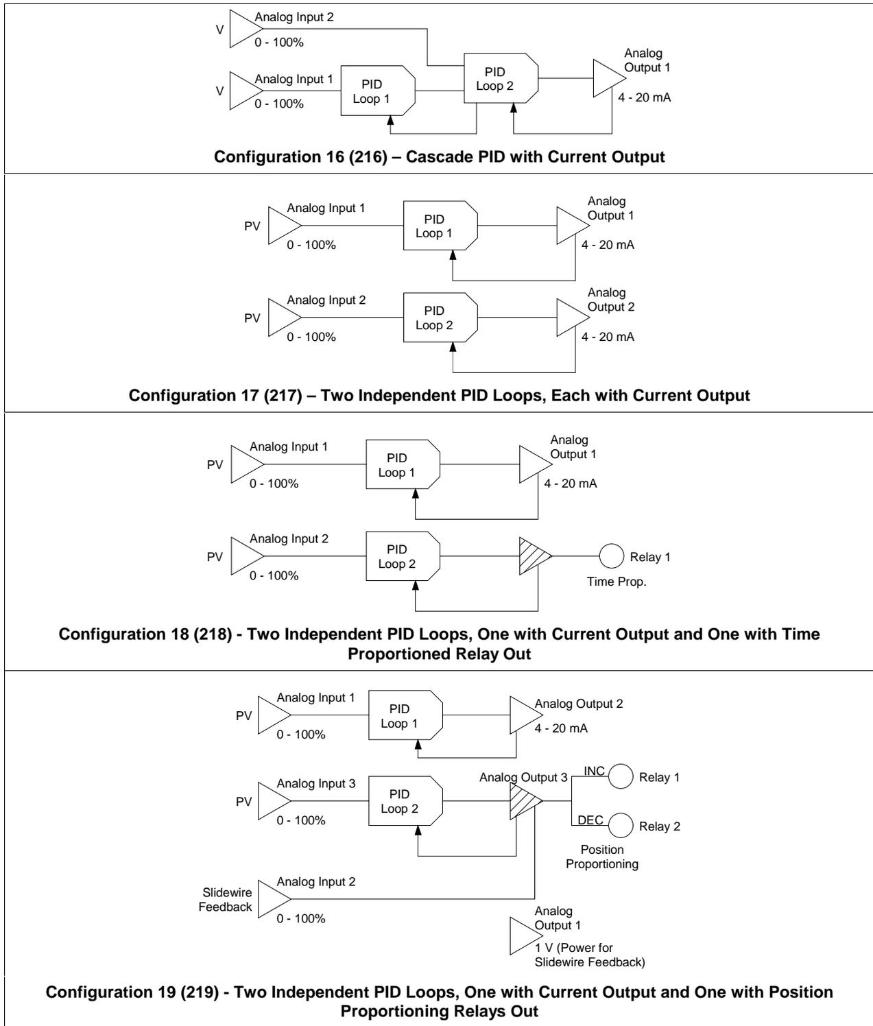
Figure 5-3 Two-Loop Factory Configurations
