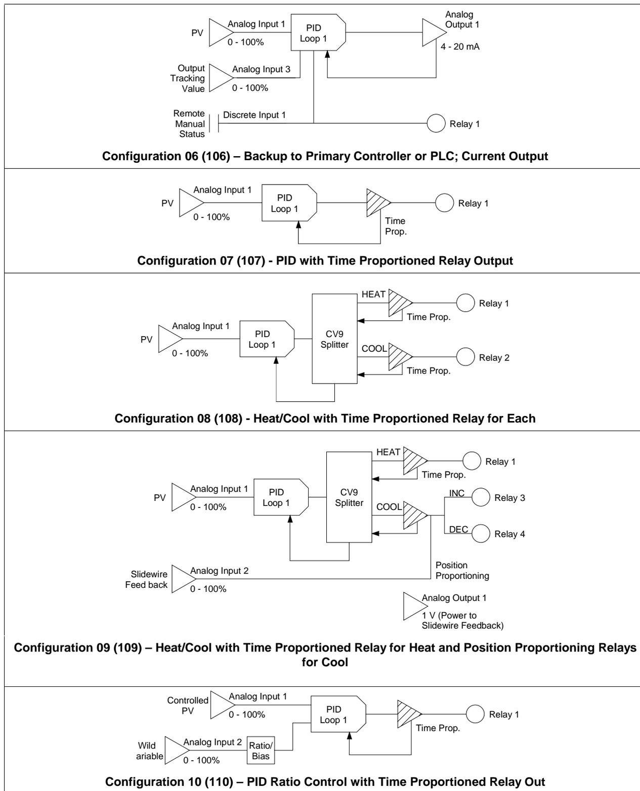
Figure 5-2 Single-Loop Factory Configurations (continued)
