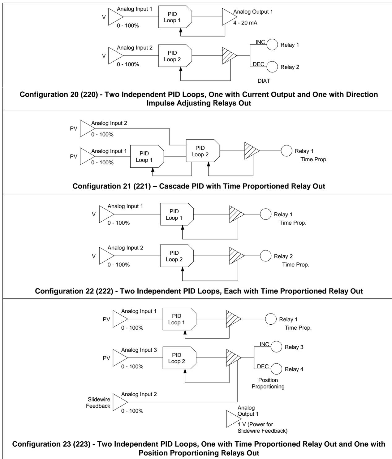
Figure 5-3 Two-Loop Factory Configurations (continued)
