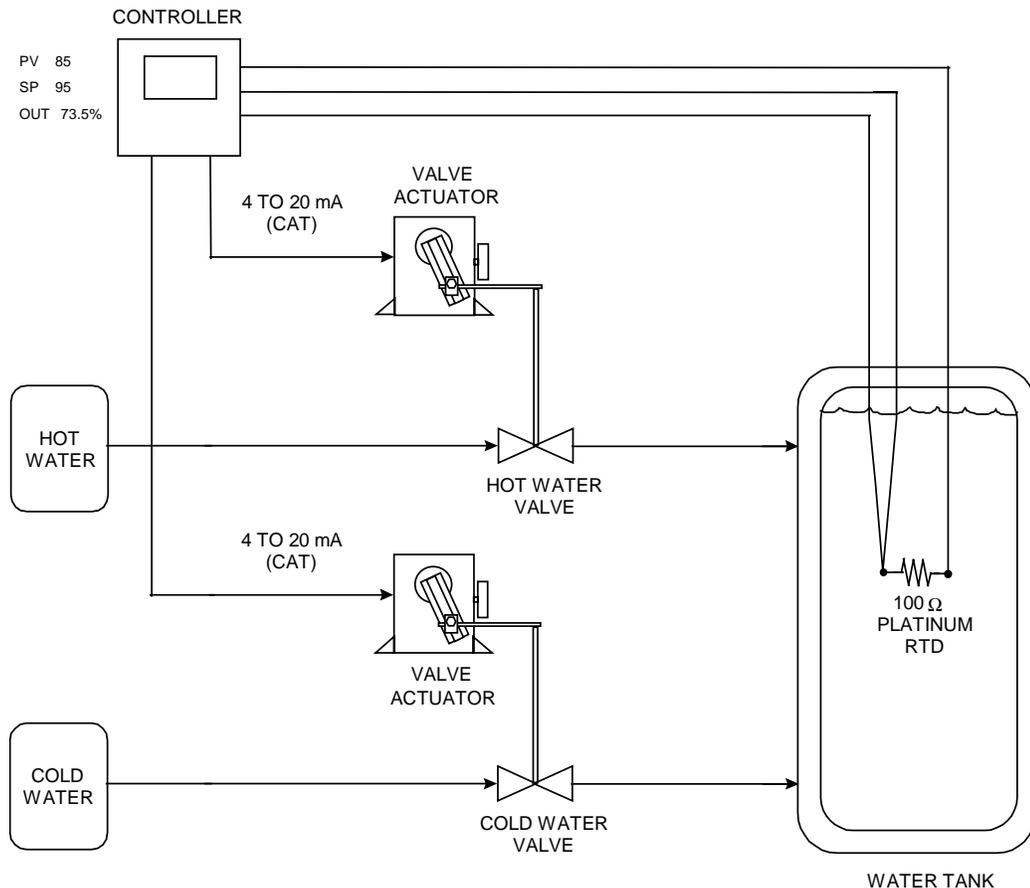
**Figure 8-9 Temperature Control of Water Using Split Output or Duplex Control**
