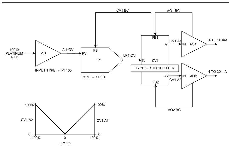
Figure 8-10 Function Block Diagram of Figure 8-9
