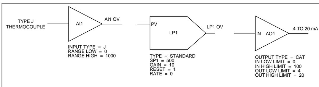
Figure 8-4 Labels for Internal Function Block Parameters
