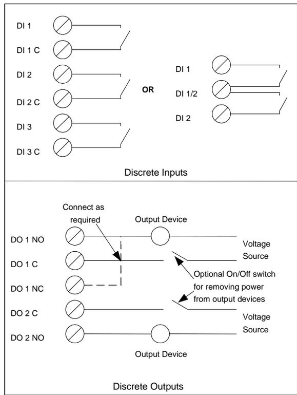
**Figure 4-7 Discrete I/O Connections**
