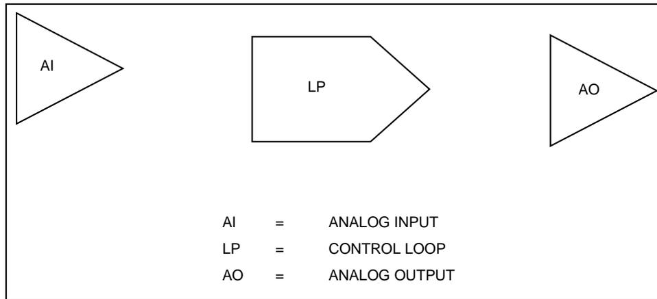
**Figure 8-2 Basic Function Blocks Required for Control Configuration of Figure 8-1**
