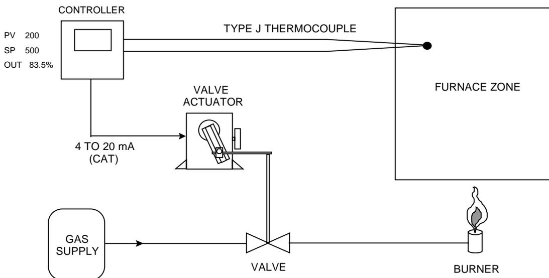
**Figure 8-1 Control of Furnace Zone Temperature with 4-20 mA (CAT) Control Signal**
