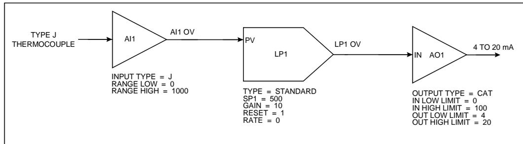
Figure 8-5 Interconnections Between Function Blocks
