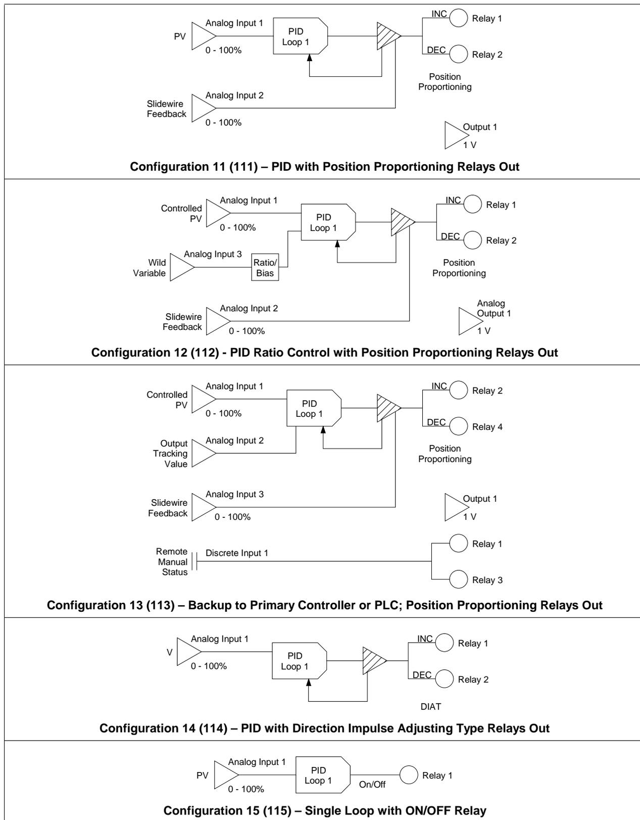
Figure 5-2 Single-Loop Factory Configurations (continued)
