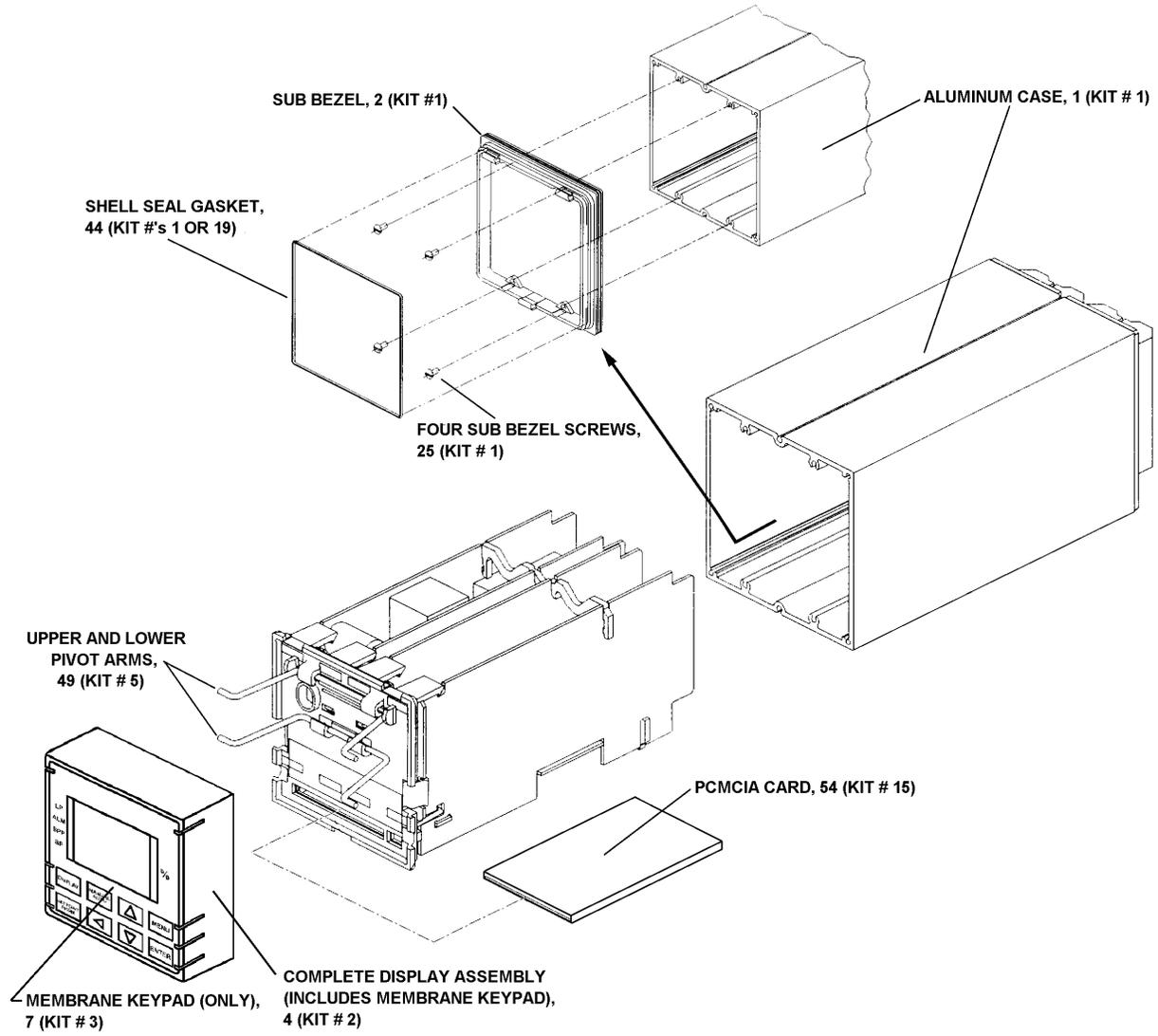
Figure 22-2 Instrument Card Cage Removed From Case along with Sub Bezel and Gasket
