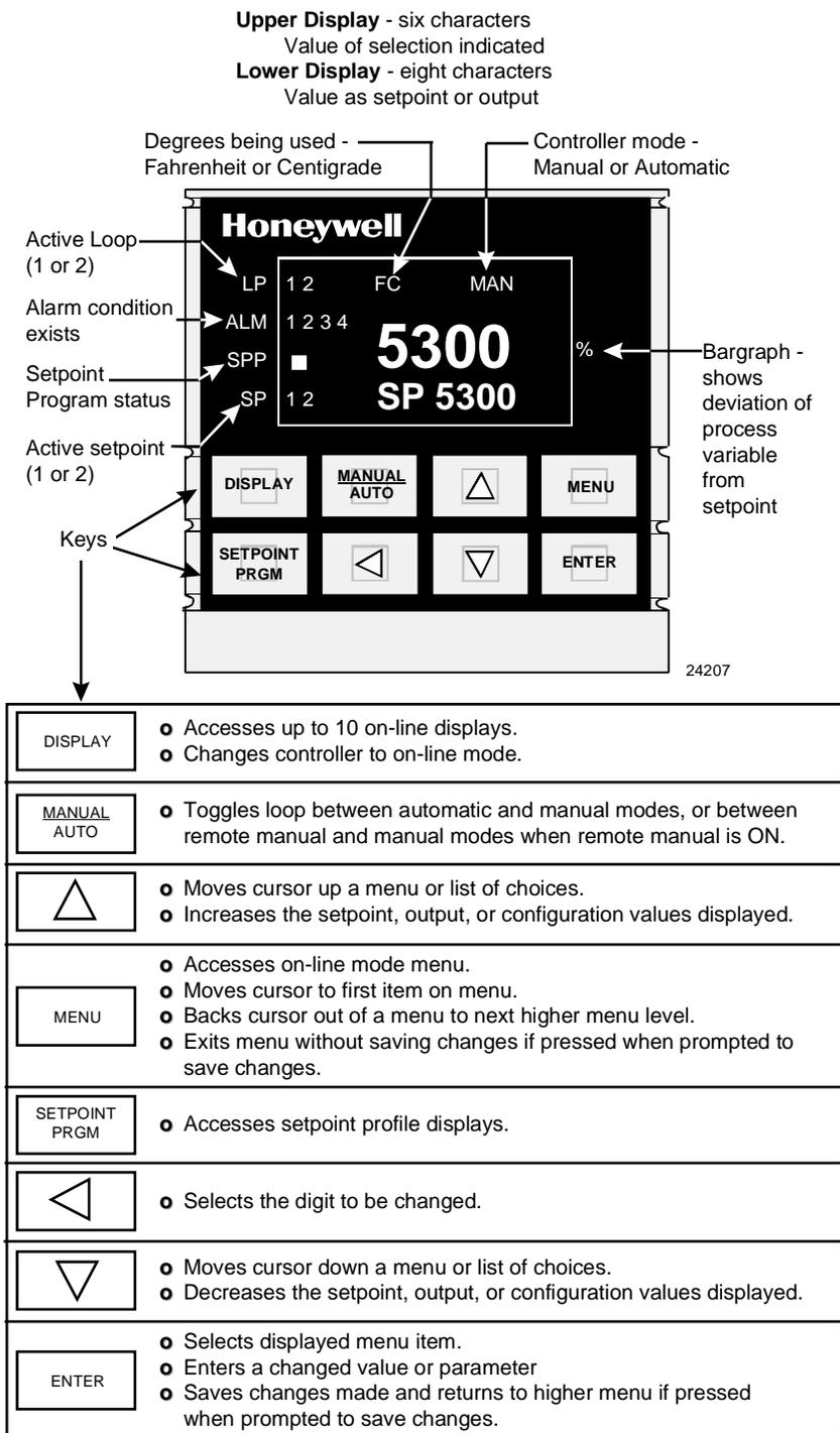
Figure 1-2 Display Indicators and Key Functions
