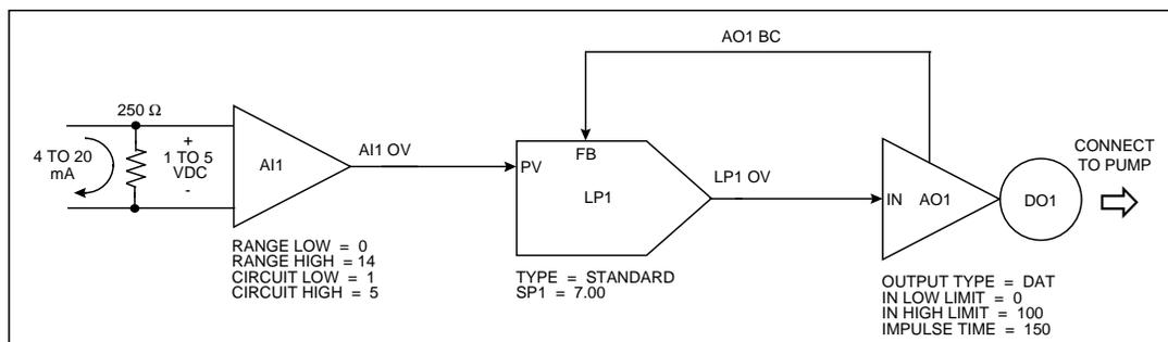
**Figure 8-8 Function Block Diagram of Figure 8-7**
