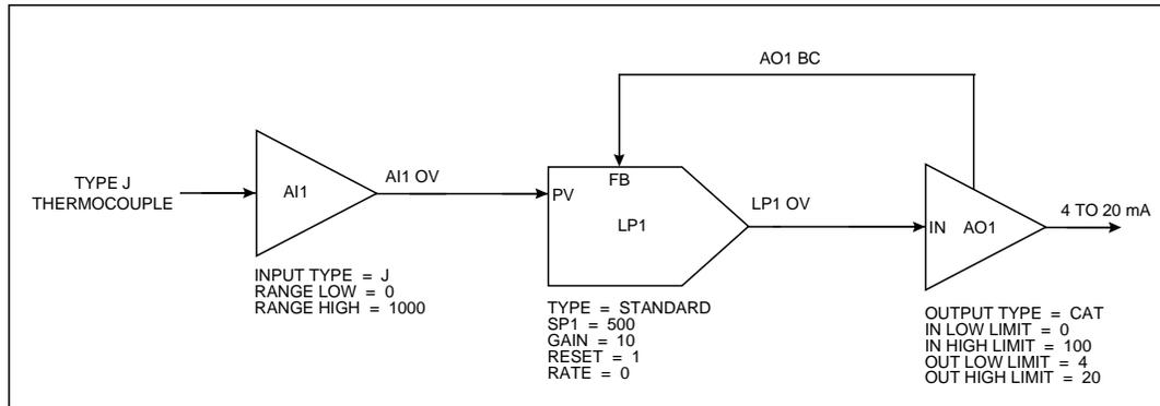
**Figure 8-6 Complete Function Block Diagram of Figure 8-1**
