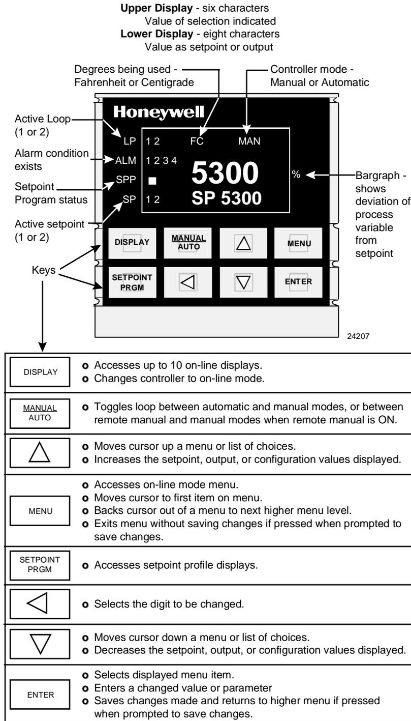
**Figure 14-1 Example Of A Primary Display**
