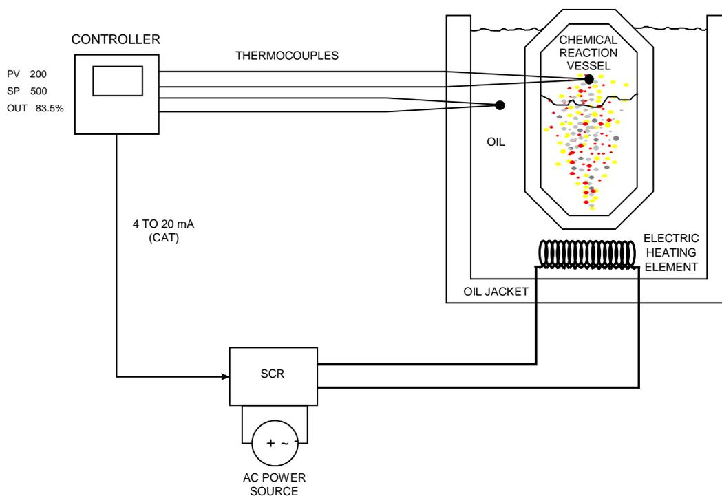
**Figure 8-11 Temperature Control of an Oil Heated Chemical Reaction Chamber**
