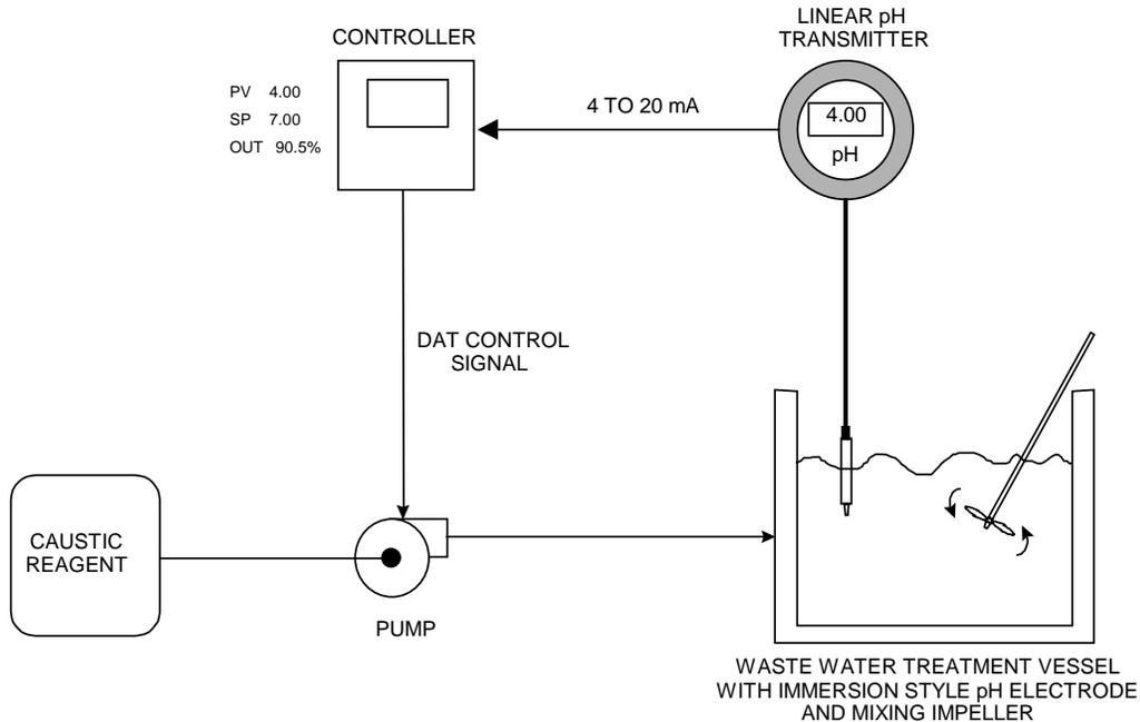
**Figure 8-7 Control of Wastewater pH Using a Time Proportioning (DAT) Control Signal**
