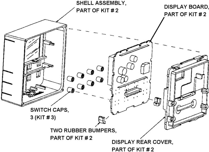
Figure 22-3 Exploded View of Instrument's Display
