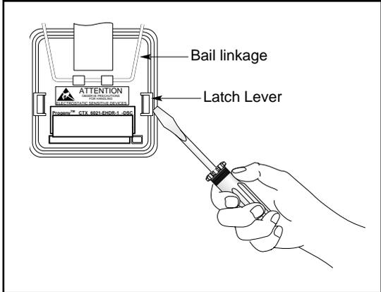
Figure 18-1 Releasing Latch Levers
