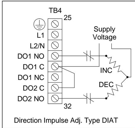
**Figure 4-9 DIAT Typical Wiring**
