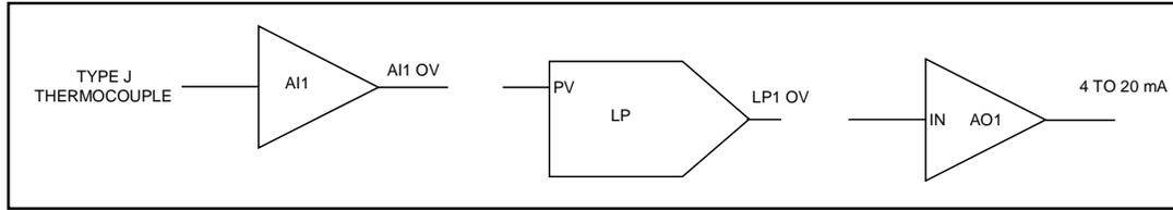
Figure 8-3 Labeling Each Function Block’s Name, and Major Inputs and Outputs
