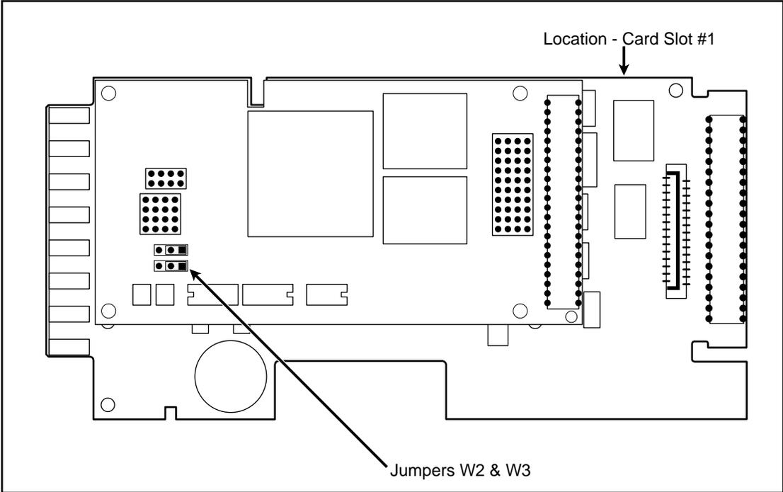
Figure 18-2 Location Of Termination Jumpers W2 And W3
