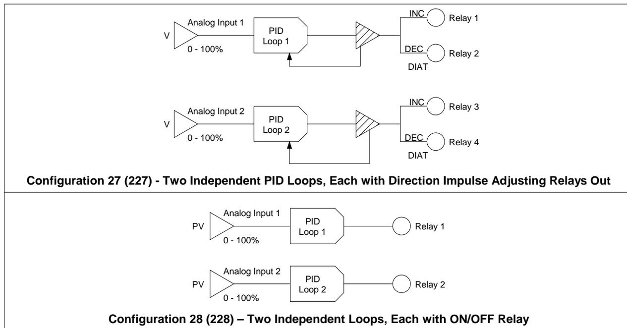
Figure 5-3 Two-Loop Factory Configurations (continued)
