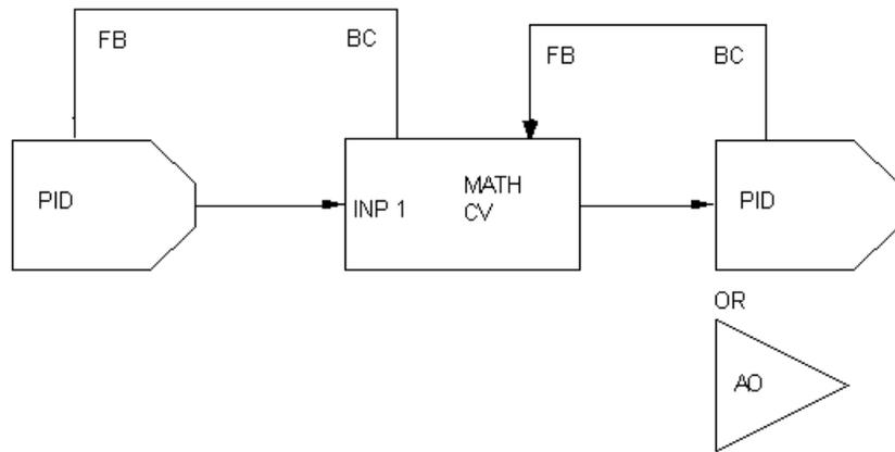
**Figure 9-1 Math CV Feedback Programming**
