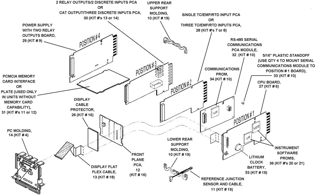
Figure 22-5 Exploded View of Instrument's Card Cage
