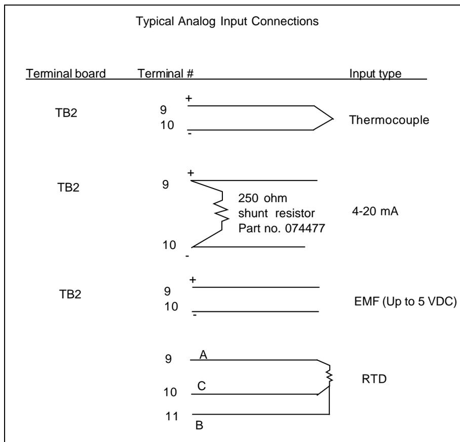
**Figure 4-6 Typical Analog Input Connections**
