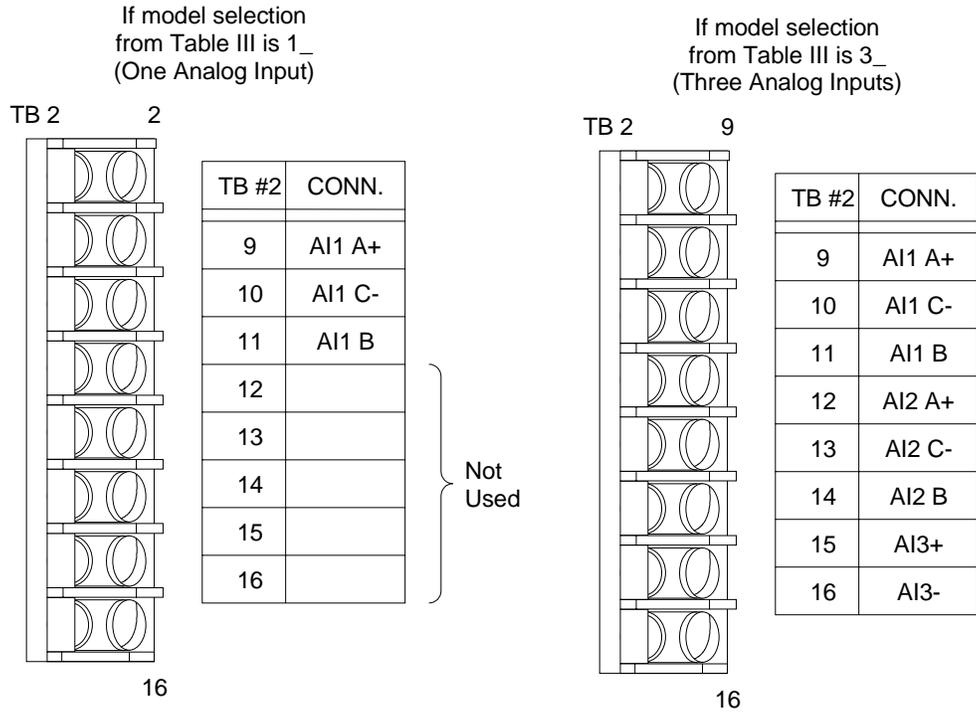
**Figure 4-3 Slot 2 Terminal Connections**
