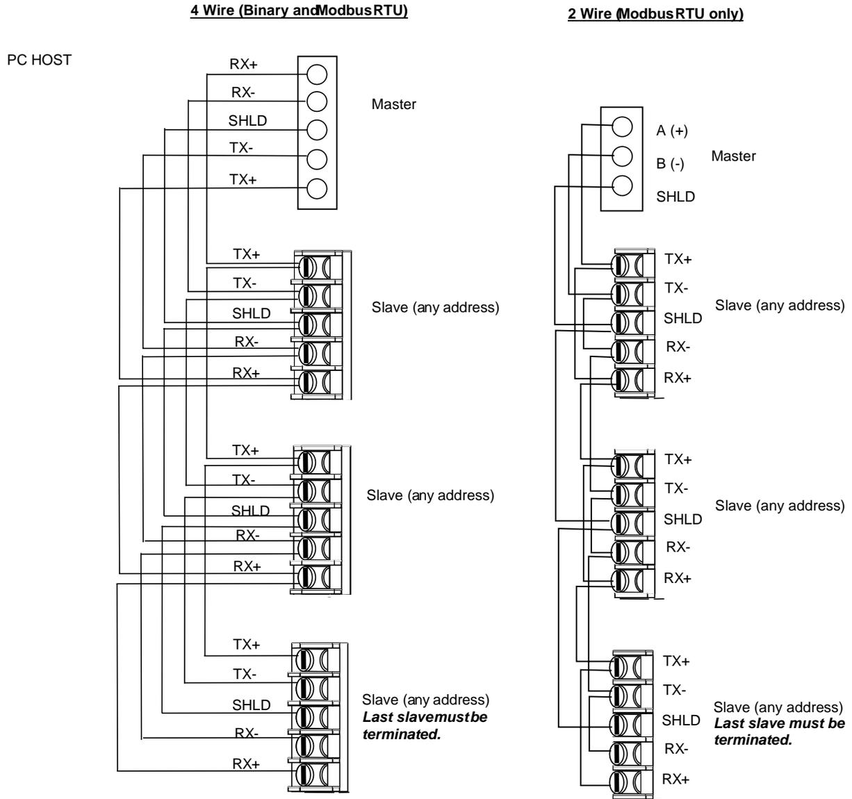
Figure 4-11 Network Data Cable Connections
