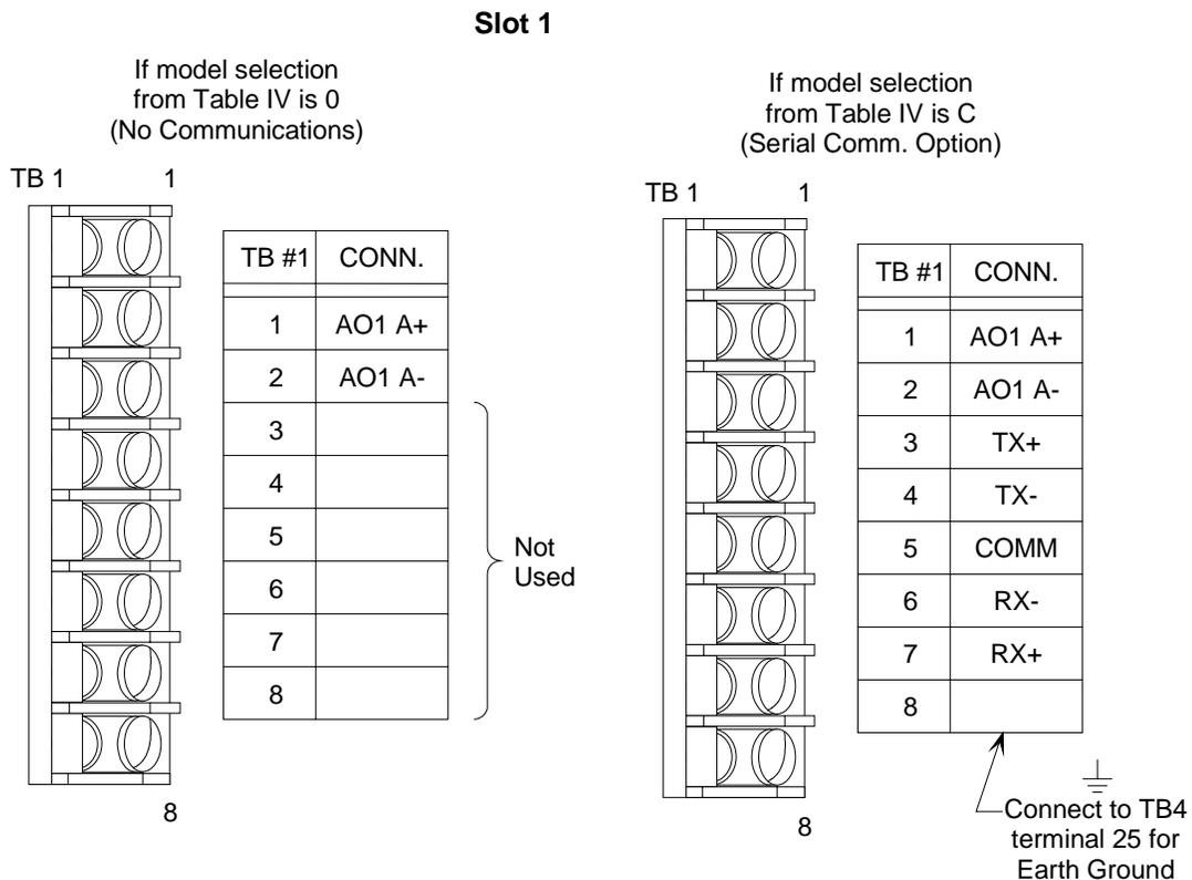
**Figure 4-2 Slot 1 Terminal Connections**
