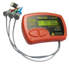
The Peak Atlas SCR is specifically designed for the rapid identification and analysis of a very wide range of thyristors and triacs. Just connect the test probes any way round and press test. The Atlas SCR will instantly identify the type of part, identify the pinout, categorise it's gate sensitivity and measure the gate voltage drop. Gate current is autoranging from 100µA to 100mA while the load test condition is maintained at 12V 100mA regardless of battery condition.
