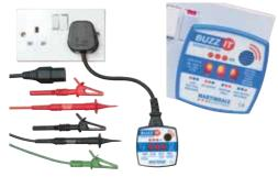
Safe and simple to use, the 'BUZZ-IT' is a real improvement for awkward sockets. It has an audible signal to tell you instantly whether or not the wiring is correct, and can also be used as a fuse finder, as the correct fuse is located when the buzzer stops. If there is a problem the pattern of neon lights indicates the fault. Any results other than three indicators lit and a continuous buzzing tone shows a fault condition.
