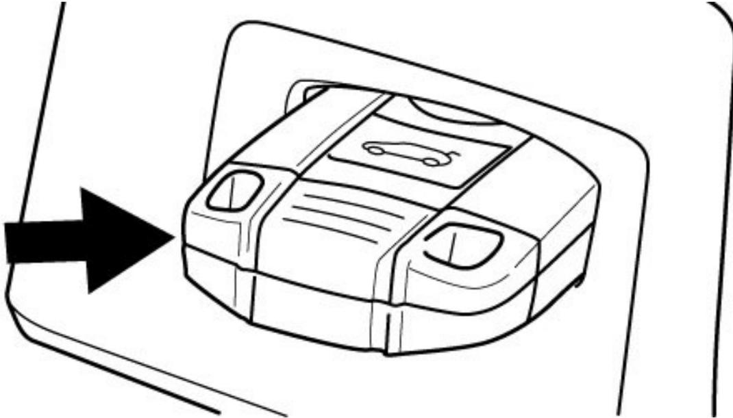
2. Locate the driver side kick panel. Remove the small plastic cover to expose the OBD-II port.
