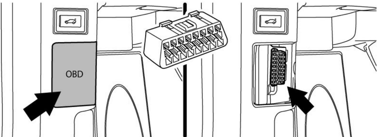
3. Plug the OBD-II cable into the OBD-II port under the dash.
