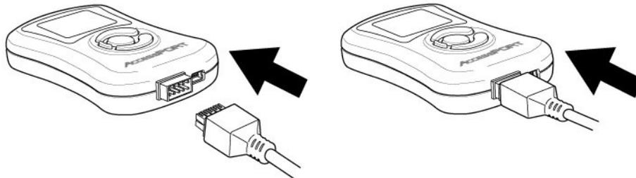
5. Make sure the clasp on the OBD-II cable firmly engages the tab on the 10-pin port.
