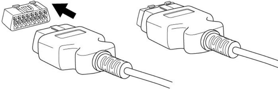
4. Connect the small end of the OBD-II cable to the 10-pin port on the bottom of the AccessPORT. At this point the AccessPORT will power up and after a few moments present the installation menu.
