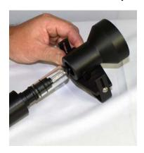
• Carefully remove the lamp cover by gently pulling it off with a twisting motion. It is best to use a glove or wrap the lamp cover with a small towel to protect your hand from accidental breakage of the glass.
