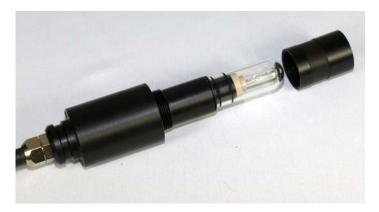
• Remove the bulb from the socket and extend it to the end of the lead wires. Carefully unplug the bulb from the wires leading into the ballast body.
