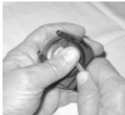
Fig. 81 -Ring Removal (alternate)
