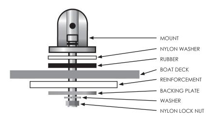
Install the tower mounts to the boat deck in the order shown in the diagram.
