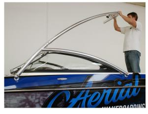
Insert the front leg hinge joint into the lower section of the front arm (repeat for the other side). Its important not to completely tighten the fittings as some adjustment will necessary before the installation is complete.
