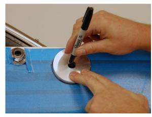
Once the desired position is achieved, place one of the backing plates over the piece of tape and trace around it with a permanent marker.
