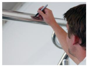
Using the pre-drilled holes in the top section tube, mark the drilling positions on the front leg tubes. We then recomend drilling the holes with a smaller drill bit (smaller than the 3/8" drill bit) to make a pilot hole.
