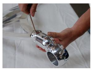
The lower section of the switch blade can now be assembled to the lower fittings and clamp using the trim washer, shoulder bolt and threaded lap joint.
