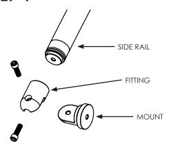
The mounting feet will need to be assembled to the side rail fittings, followed by attaching them to the side rails.
