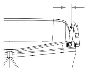
Measuring from your windshield, check the distance to the side rail to make sure both sides are symmetric.
