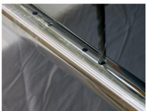
Following the pilot holes you just drilled, use a 3/8" drill bit to create the clearance hole for the joining bolts. As each hole is drilled we recommend inserting each bolt so that it keeps the parts aligned while drilling the next hole.
