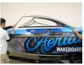
Once the feet are connected to the side rails, hold the side rail up to your boat. Once the rail is aligned with your windshield use a small piece of tape to mark the position of the mounting feet.
