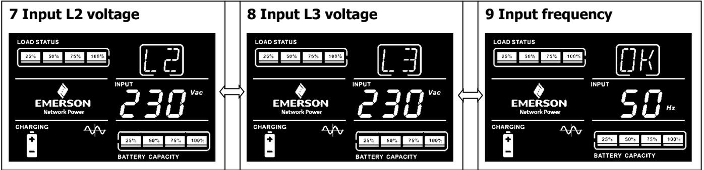
**B. Parallel model:** Compared to single model, parallel model will have one more screen to display parallel information of UPS unit.
