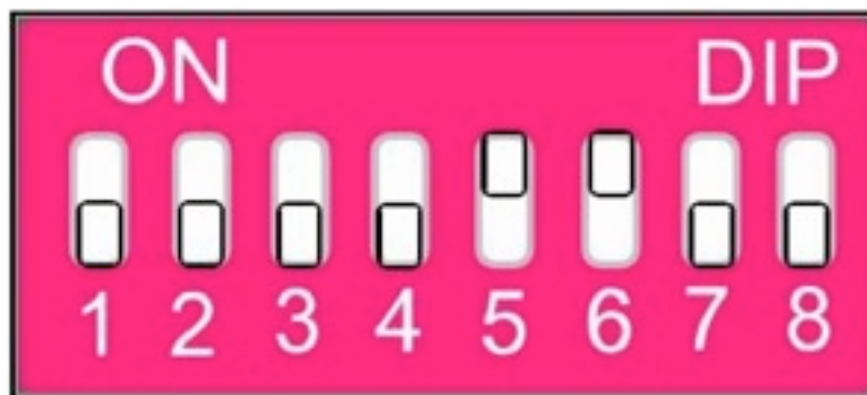
DIP switch setting for Right Mix Mode (00001100). Exponential and MCU Mode are turned off.
