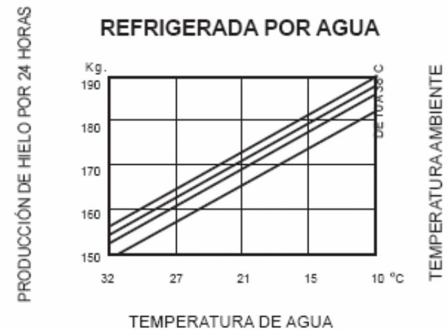
**NOTE:** The daily production capacity change when the environmental temperature and the water supply change, a capacidad de producción diaria varía al variar la temperatura ambiente y del agua de alimentación, thus the space around the equipment.. So as to maintain the equipment in maximum efficient conditions, it is necessary to do the periodic maintenance as explained in the correspondence part of the manual
