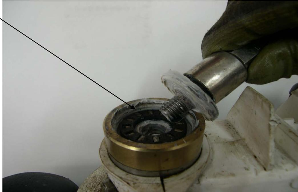
1. CLEAN THE OLD GREASE WITH A RAG AND OIL 6 IN 1, TO GREASE THE BEARING WITH GREASE OF "ALIMENTATION AND WATER REPELENT".
