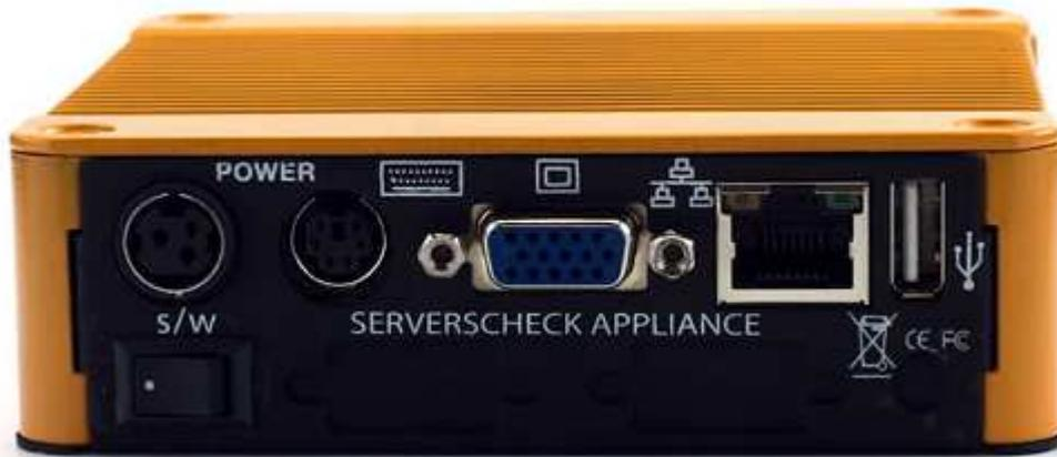
On the back of the appliance you can connect a monitor using a standard VGA cable, a PS2 keyboard and a mouse. If you don't have a PS2 keyboard then you can also use an USB keyboard using the USB port on the front. When connected you will be prompted with a standard windows login screen as shown below.
