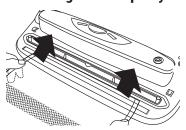
3. Close Lid. Position hands on both sides of the Lid. Press firmly on both sides of the Lid and hold until the motor starts.
