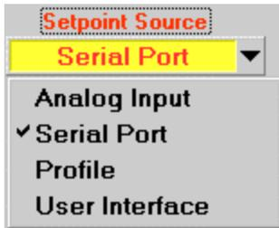
**Analog Input** - The setpoint is to be obtained from the controller's analog input (4 to 20 mA or 1 to 5 V analog signal).
