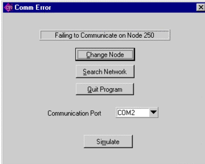
This window will appear if the controller is not properly wired to the computer or if the wrong node number has been selected.
