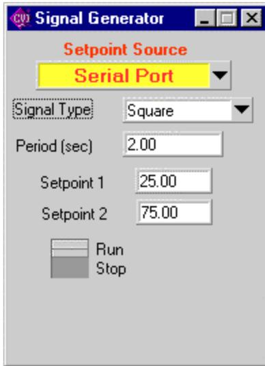
The setpoint source gives the user the ability to determine where the setpoint comes from. The four options are:
