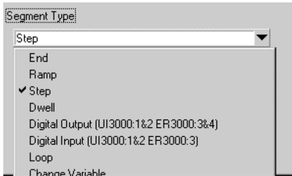
An "**End**" segment is used to end the profile.
