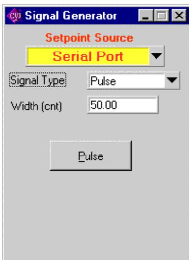
[Note however, that the controller will still attempt to perform it's normal PID algorithm even when the signal generator is in pulse mode (to overcome this set the Proportional and Integral min/max terms to zero to disable PID control).]
