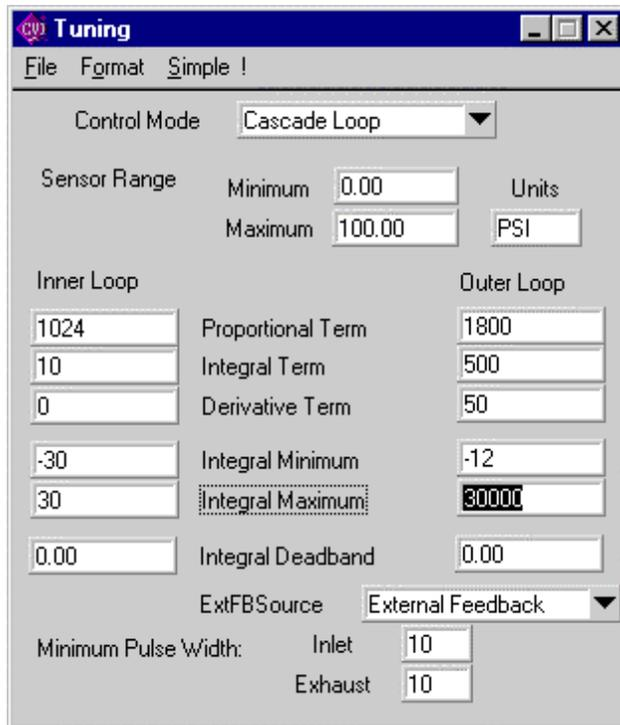
The menu item labelled **Simple** (toggles to **Advanced**) reduces the number of parameters displayed and is useful for inexperienced users.
