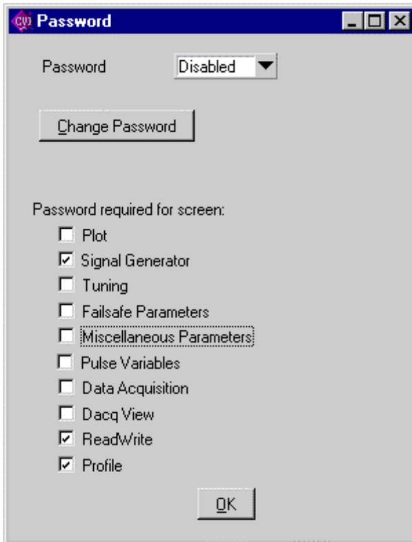
To enable the password the first item must be selected to "Enable".
