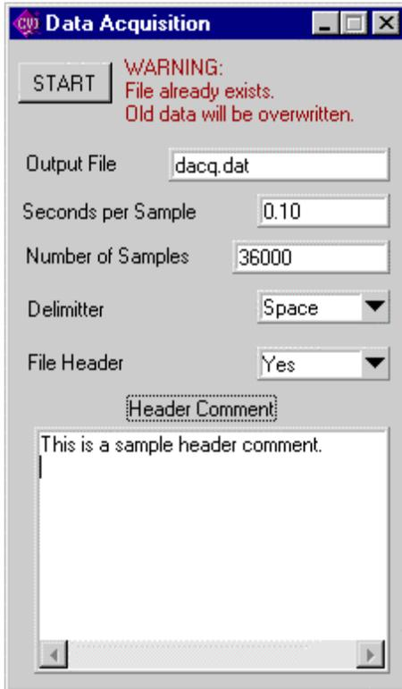
An optional file header can be written to the start of the file which includes the date and time and a user specified comment. Delimiters between data (data includes the time, with a resolution of .001 seconds, the setpoint and the feedback) can be specified as spaces, tabs or commas.
