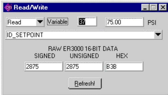
Each screen is set up for either reading or writing via the parameter in the upper left hand corner of the screen.
