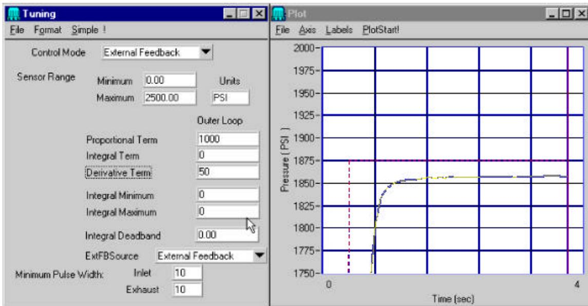
What can be done to eliminate the offset is the addition of integral term. The resulting response follows:
