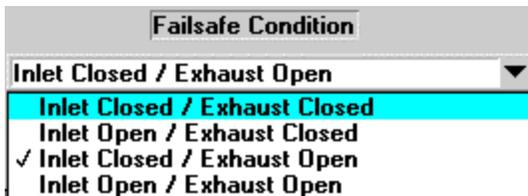
Normally, "Inlet Closed/Exhaust Open" should be selected so that the controller vents to atmosphere if a failsafe limit is exceeded.
