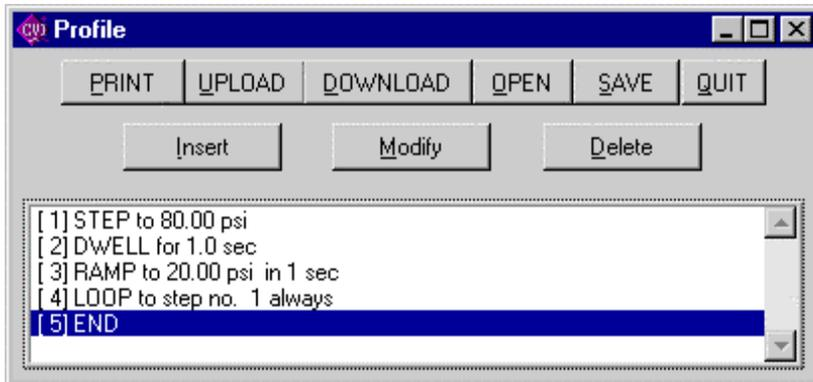
The **PRINT** outputs the profile to a printer. **UPLOAD** reads the profile from the controller and displays it on the screen (upload also takes place automatically when the window is opened). **DOWNLOAD** writes the newly created or modified profile into the controller. **OPEN** reads a profile from a file. **SAVE** writes a profile to a file. **QUIT** closes the profile window.
