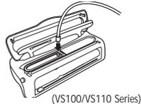
3. Attach other end of the Accessory Hose to the Accessory Port on the Canister Lid.
