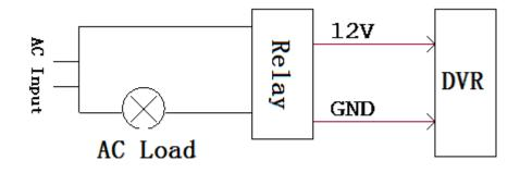
The connection diagram of alarm output as following:
