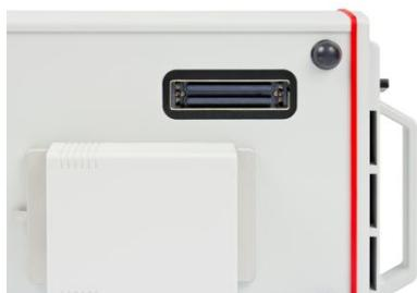
*Fig. 12 Probe socket (port) at the back of the device*
