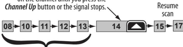
The radio scans about 5 channels in 0.5 seconds.
