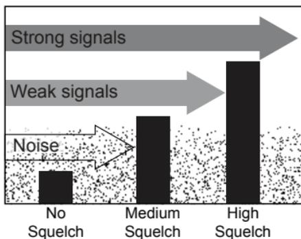
To adjust the squelch level, press and hold the **VOL SQL** key. The screen displays SQL and a SQUELCH level number (0 - 3). Use the **Channel Up** and **Channel Down** keys to adjust the squelch level. Press and hold the **VOL SQL** key again to set the squelch level and return to the main display.
