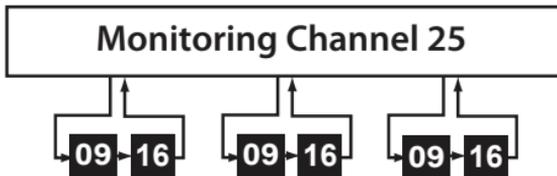
Every two seconds, the radio checks channels 9 & 16.
