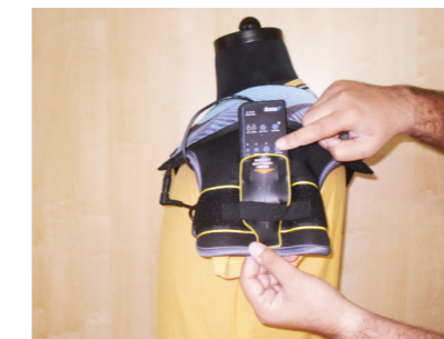
Step 8: Set the required temperature and mode with the help of CLIMAWARE™ Rx Touch Controller + Battery Unit. Please refer to sections 'How to charge the battery' and 'How to use CLIMAWARE™ Rx Touch Controller'.
