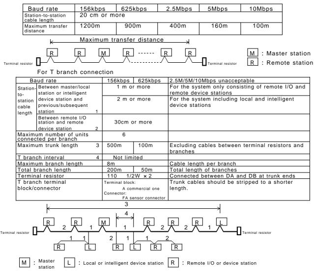
Note: All units and cables on the system should be compatible with the CC-Link, Ver. 1.10.
