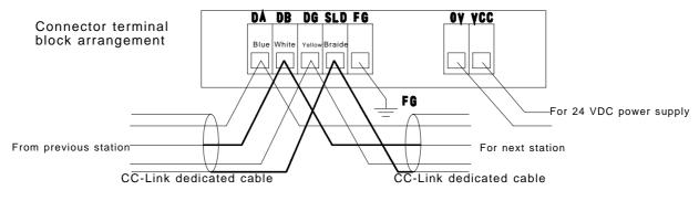
Each cable should be stripped to 7 mm.
