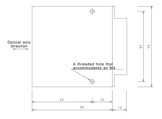
Note 1: Tighten the C remote SOT mounting screws to a torque not higher than 8 kgf-cm.
