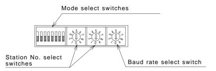
4-2-1.Setting the station No. select switches Station No. select switches
