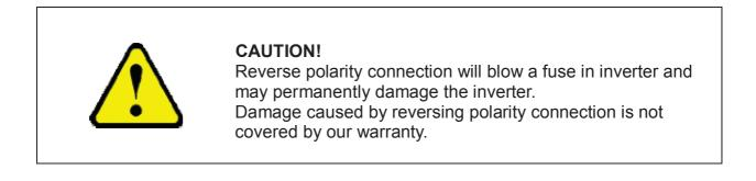
2-4-4 Connect the cable from the negative terminal of the inverter to the negative terminal of the power source. Make a secure connection.
