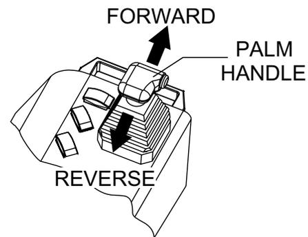
Figure 15. Left Joystick Control
