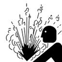
**HOT** coolant can cause severe burns. **DO NOT** remove cap if radiator is **HOT**.
