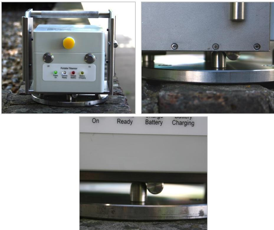
For Horizontal Tilt-Plates, place the Tiltmeter on the Tilt-Plate and ensure that the locating bars touch the protruding rounded studs on the Tilt-Plate *in both directions* (see photos above).
