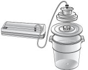
Close the lid. Lock the lid by pressing in the locks on both sides. (You may need to press down lightly on the stars while pressing in the locks.)
