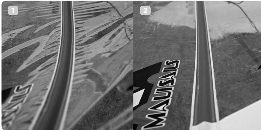
Pic. 1 - Visible wrinkles. Pic. 2 - Smooth area after some batten tension applied
