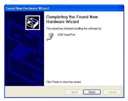
Click on the finish button. The drivers are now installed. Please note that you will not need to repeat this procedure unless the drivers are uninstalled.
