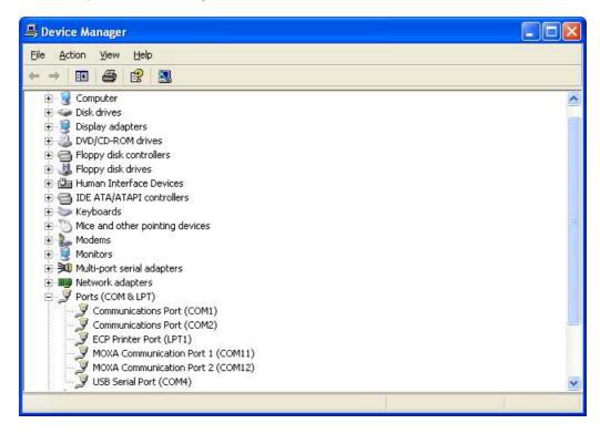
The port number is in brackets after the text USB Serial Port, (COM4) in the example above.
