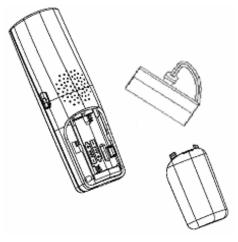
Place the handset in the base station to charge for 16 hours prior for first use. If you don't properly charge the phone, battery performance will be compromised.
