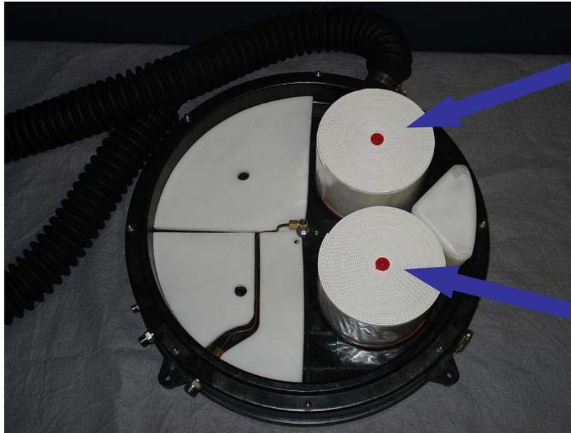
**Warning:** Do not attempt to breathe the SCBA with only one CO2 cartridge installed. Failure to install two new CO2 cartridges will result in high levels of CO2 and may lead to serious injury or death. Breathing the SCBA with CO2 cartridges that have been previously used or expired may cause serious injury or death.
