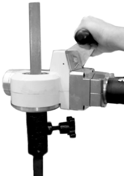
*Figure 5-4. Slide the WAVE™ handheld system down onto the valve key and rest it on the stop collar.*
