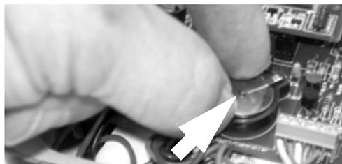
Figure 7-11. Slide the new battery into the socket, with the plus side (+) up.
