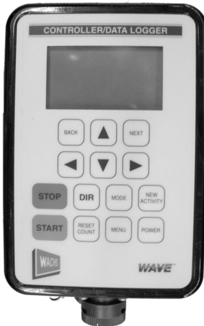
Figure 3-7. VITALS™ controller/data logger
