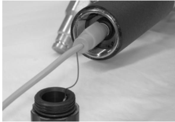
*Figure 3-12. Charger plugged into the battery charging connector. Note that the connector must be aligned correctly to line up the pins with the sockets.*
