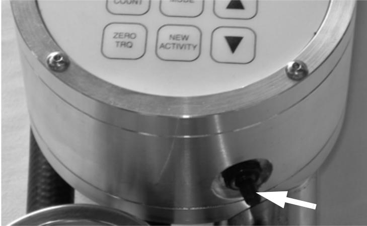
*Figure 7-7. Control unit power switch (hydraulic and pneumatic systems only). Press the button and release it to toggle the control unit on and off.*
