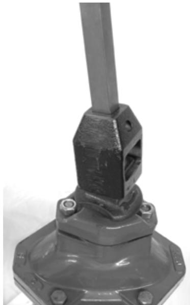
*Figure 5-2. Put the socket onto the valve nut.*
