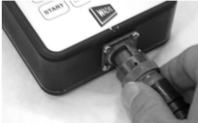
*Figure 3-19. Plug the charger cable into the VITALS™ connector.*
