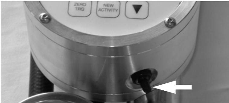
Figure 5-9. Press the power button on the control unit to turn it on.
