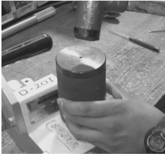
*Figure 7-5. Tap the seal into place with a hammer until the sleeve is flush against the housing.*
