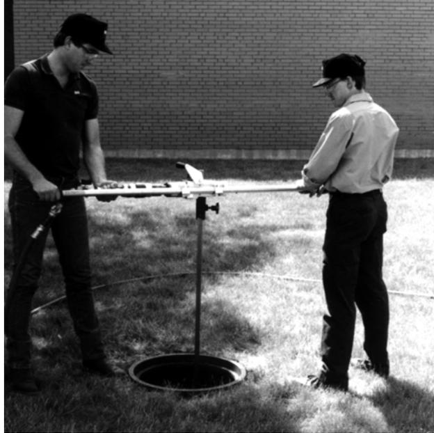
Figure 5-27. Operating the WAVE™ handheld system in two-person mode.
