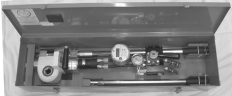
*Figure 3-24. WAVE™ handheld system in its storage case.*
