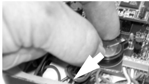
Figure 7-10. Remove the old battery from the socket.
