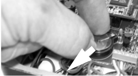
*Figure 3-17. Remove the old battery from the socket.*
