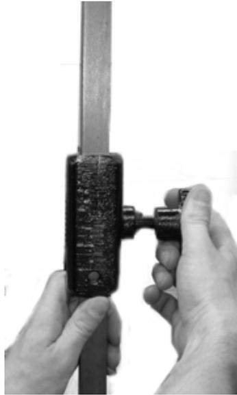
*Figure 5-3. Slide the stop collar onto the key and use the set knob to fasten it at an appropriate height.*
