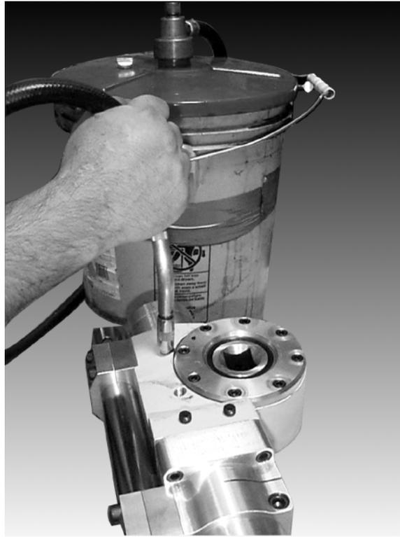
*Figure 6-2. Adding oil to the gearbox.*
