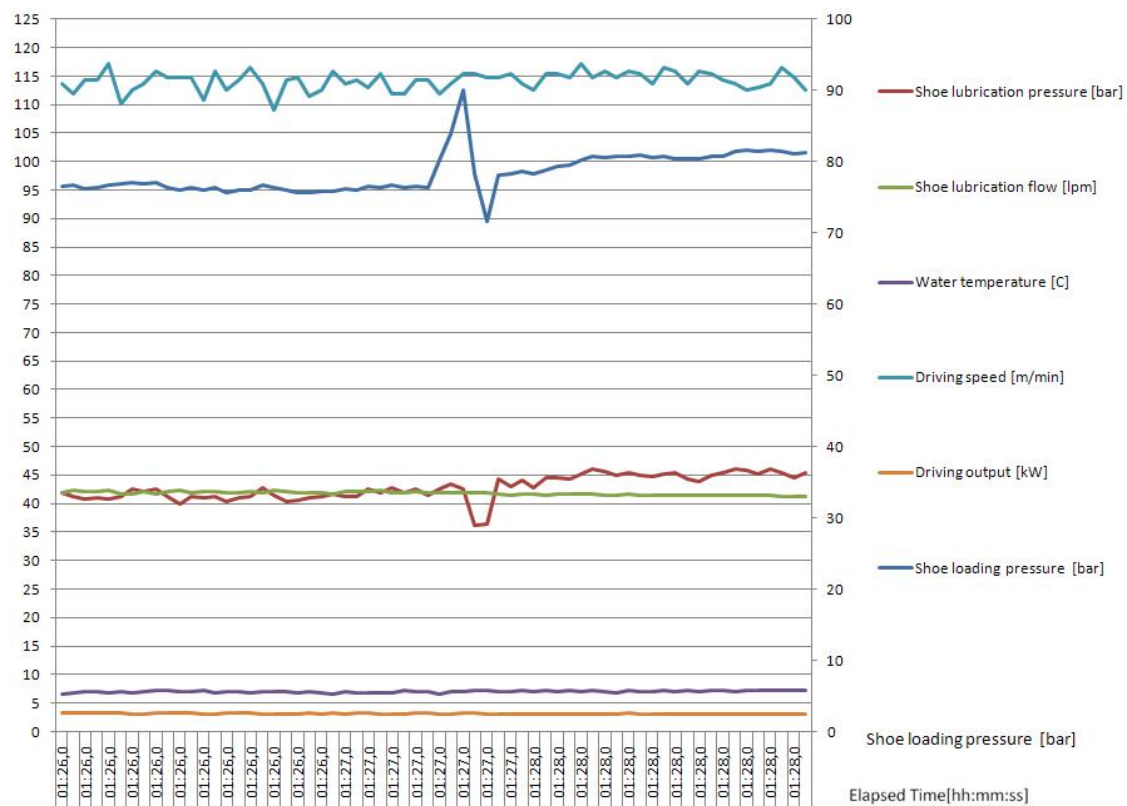
Figure 66 Shoe loading pressure 80 bar, 1600 g/m 2 wad in the time line from 86 to 88 seconds
