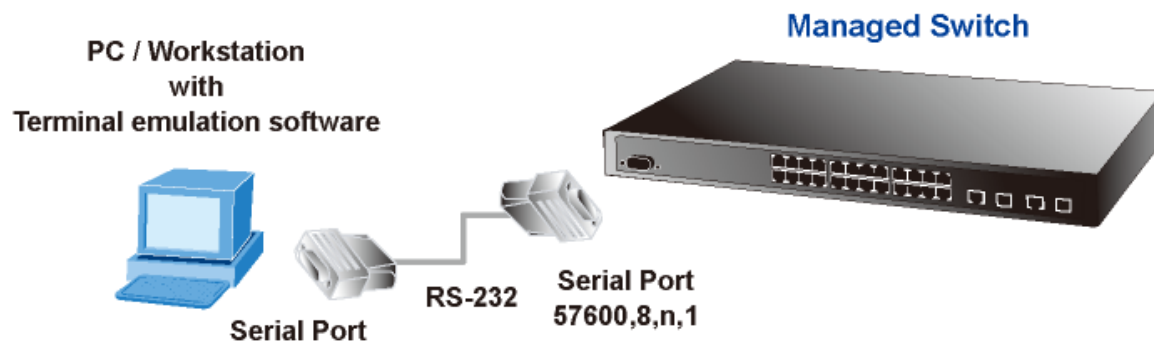
Figure 3-4: Console management setup
