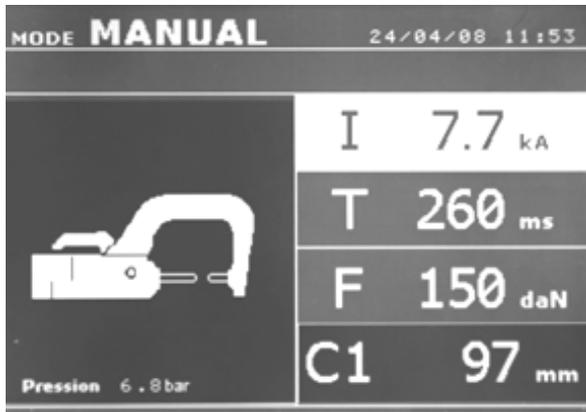
The settings proposed by default in the manual mode correspond to the settings automatically selected by the standard mode (thickness and type of sheet, electrode force, arm).
