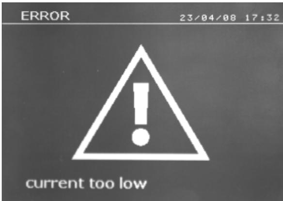
If the welding current obtained during the welding spot is 6% less than the current setting, the machine displays, once the welding spot is performed, an error message "Current too low", warning that the welding spot should be checked.
