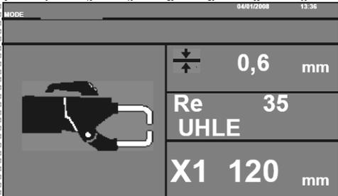
This mode is identical to the standard mode, except that the user can define the elasticity limit of the sheet. This limit (Re) can be identified using a metal tester like Gysteel Vision.
