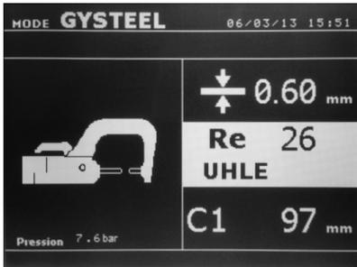
This mode is identical to the standard mode, except that the user can define the elasticity limit of the sheet. This limit (Re) can be identified using a metal tester like Gysteel Vision.
