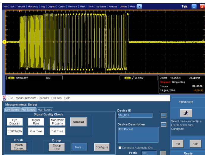
Measurement Select menu for the Signal Integrity test.
