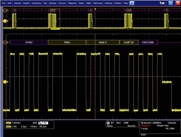
Color-coded decoded display of low-speed USB bus, showing Sync, PID, CRC, and Stop components of the serial signal.
